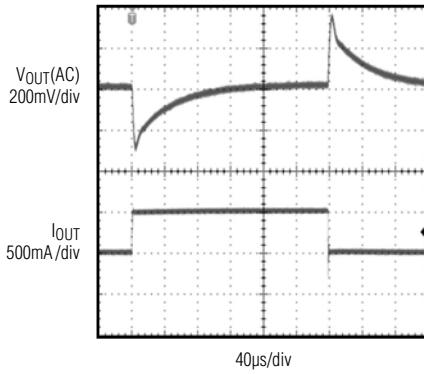
Figure 5. MAX17502G 500mA to 1A Load Transient
