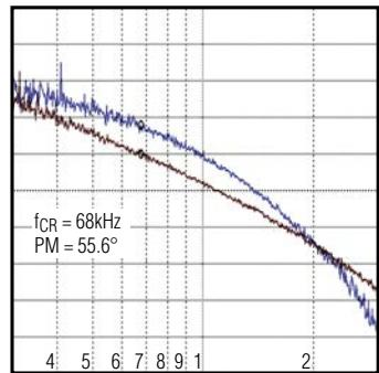
Figure 3. MAX17502G Full-Load Bode Plot ( $V_{IN} = 24V$ )
