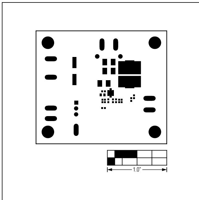
Figure 10. MAX17502G EV Kit Component Placement Guide—
