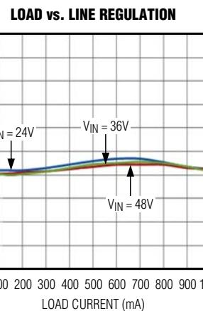
Figure 1. MAX17502G Load and Line Regulation
