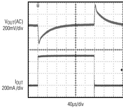
Figure 4. MAX17502G No Load to 500mA Load Transient
