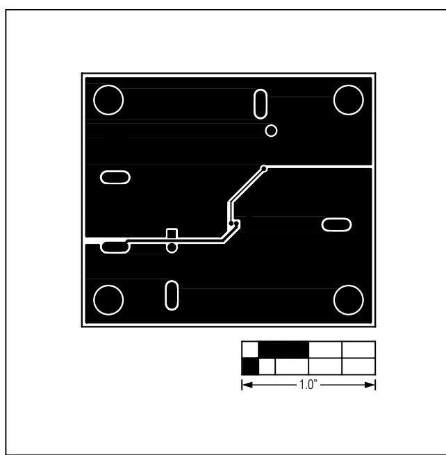
Figure 9. MAX17502G EV Kit PCB Layout—Solder Side
