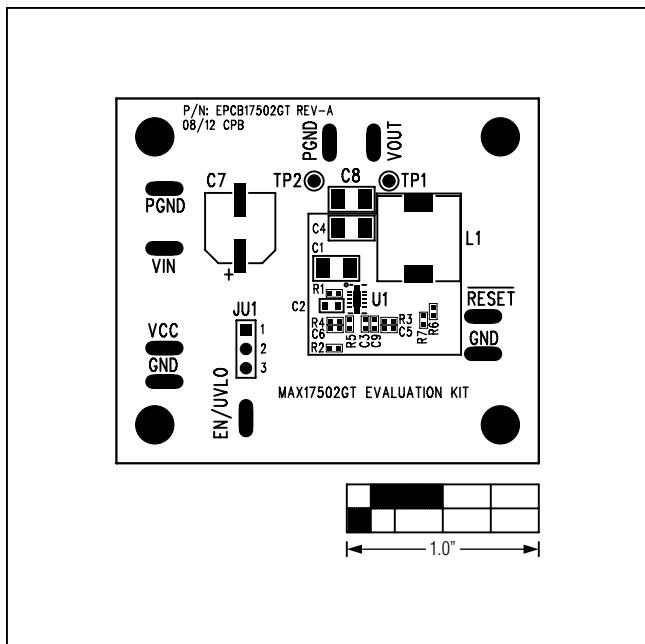
Figure 7. MAX17502G EV Kit Component Placement Guide—Component Side
