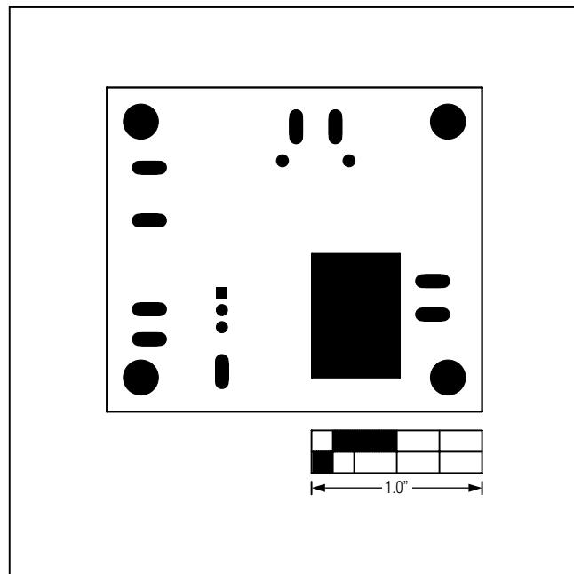
Figure 11. MAX17502G EV Kit Component Placement Guide—
