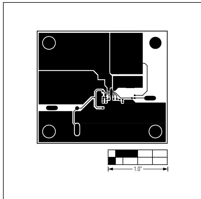
Figure 8. MAX17502G EV Kit PCB Layout—Component Side
