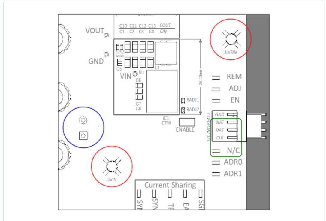
Figure 4. Optional Test Points & Component Locations
