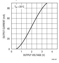
Driver Output High Voltage vs Output Current
