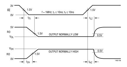
Figure 8. Receiver Enable and Disable Times
