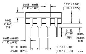
\*THESE DIMENSIONS DO NOT INCLUDE MOLD FLASH OR PROTRUSIONS. MOLD FLASH OR PROTRUSIONS SHALL NOT EXCEED 0.010 INCH (0.254mm).
