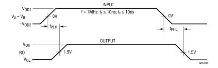
Figure 7. Receiver Propagation Delays
