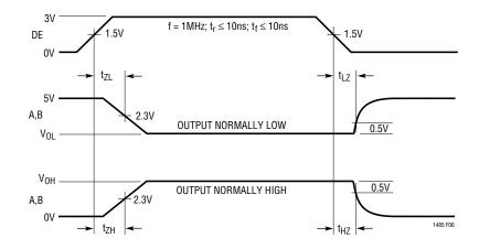
Figure 6. Driver Enable and Disable Times
