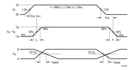
Figure 5. Driver Propagation Delays
