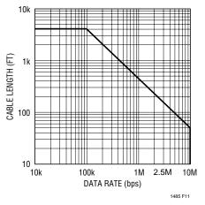
Figure 11. Cable Length vs Data Rate
