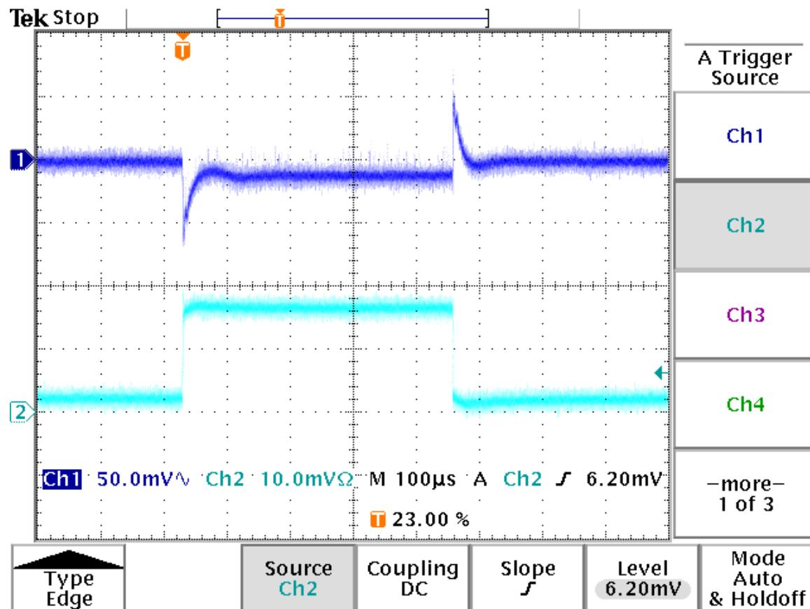
**Figure 3. Load Step Response**
