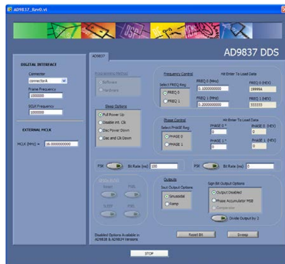
Figure 29. AD9837 Evaluation Software Interface
