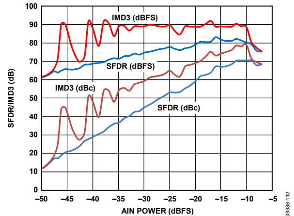
Figure 12. Two-Tone SFDR/IMD3 vs. Input Amplitude (AIN) with f_{IN1} = 29.1 MHz and f_{IN2} = 32.1 MHz
