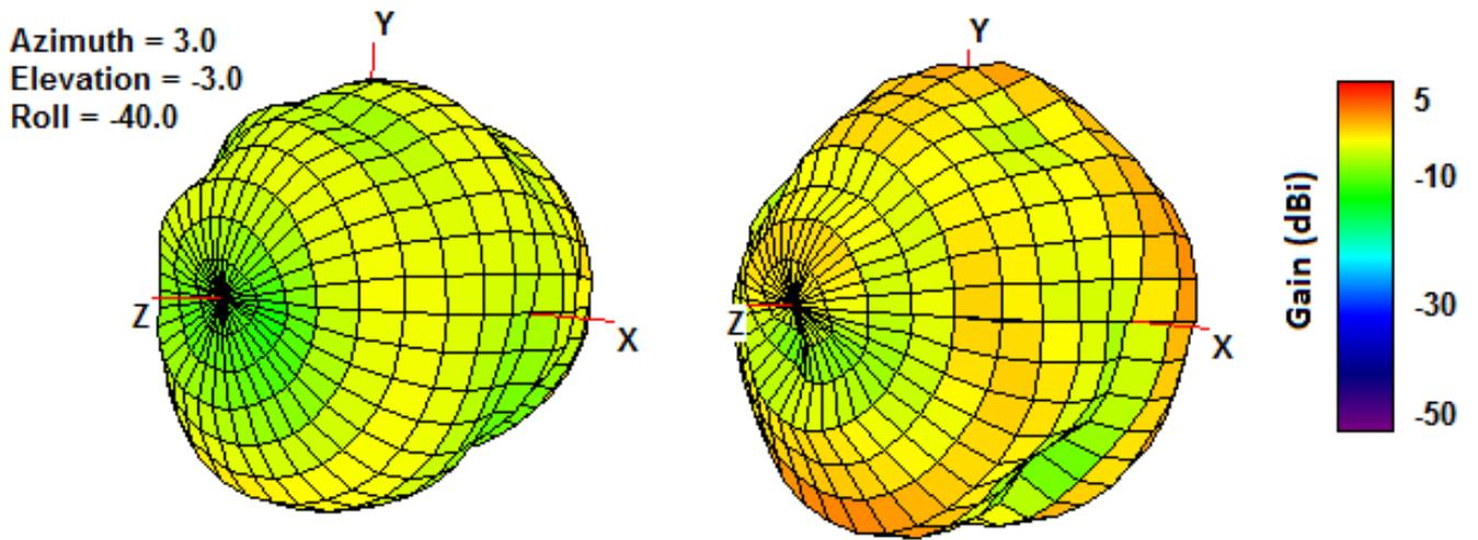
**Figure 12.** 3D Radiation Pattern at 2450 MHz (left side), Radiation Pattern at 5000 MHz (right side) of the FXP840 Antenna.
