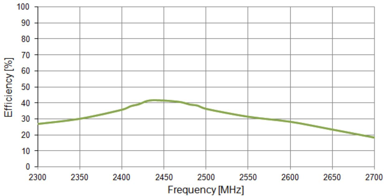
**Figure 6.** Efficiency of the FXP840 antenna from 2300 MHz to 2700 MHz.
