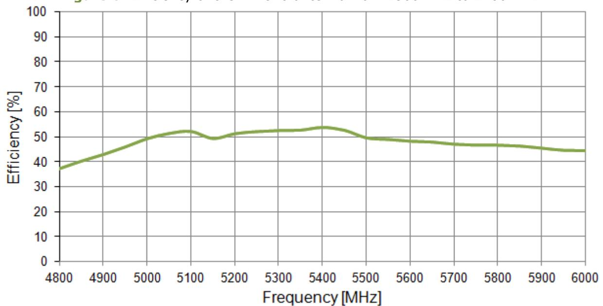
**Figure 7.** Efficiency of the FXP840 antenna from 4800 MHz to 6000 MHz.
