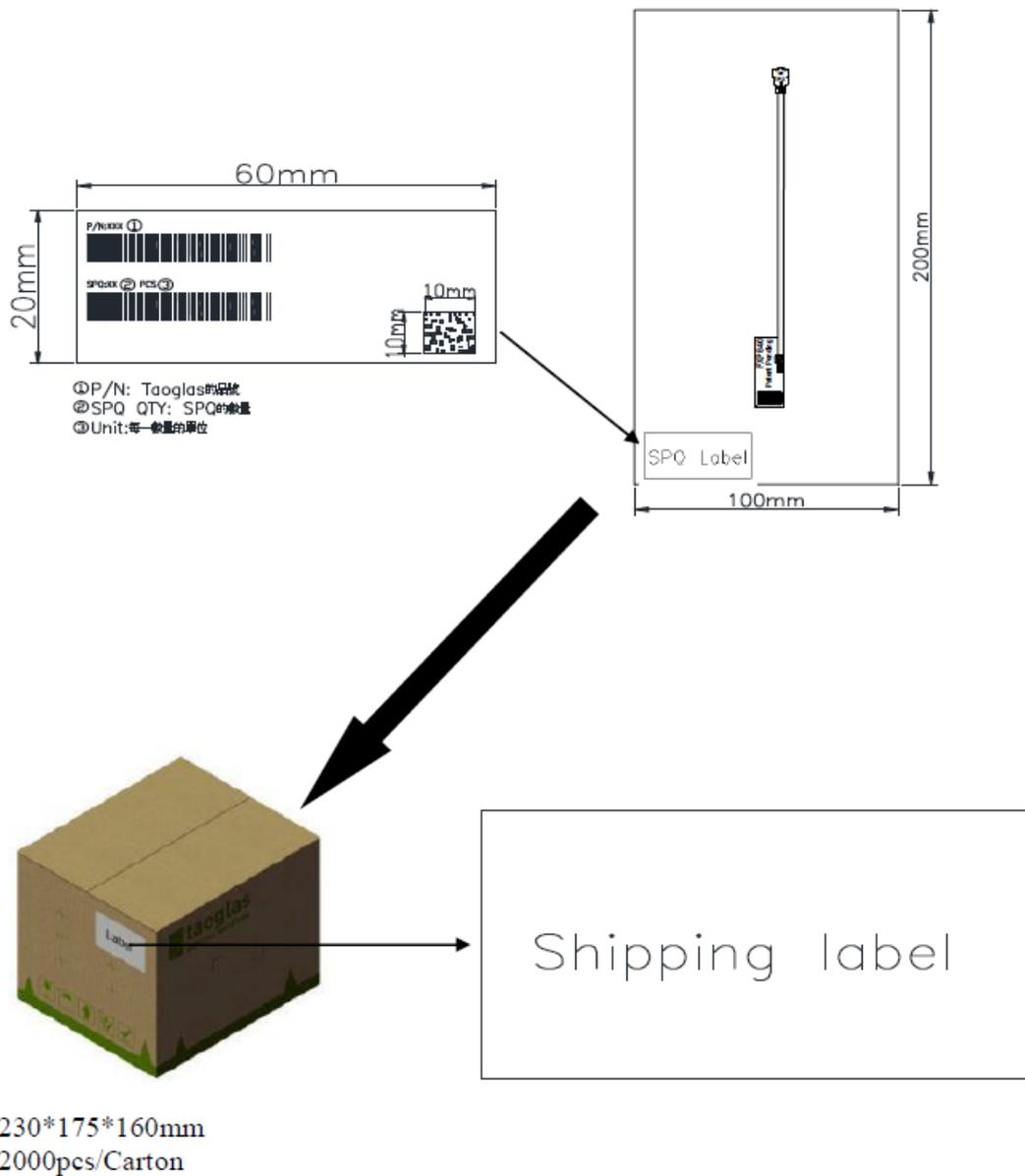
**Figure 16.** Package of the FXP840 Antenna.
