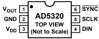
Figure 3. SOT-23 Pin Configuration
