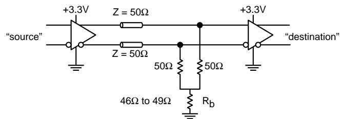
Figure 2. Three-Resistor "Y-Termination"
