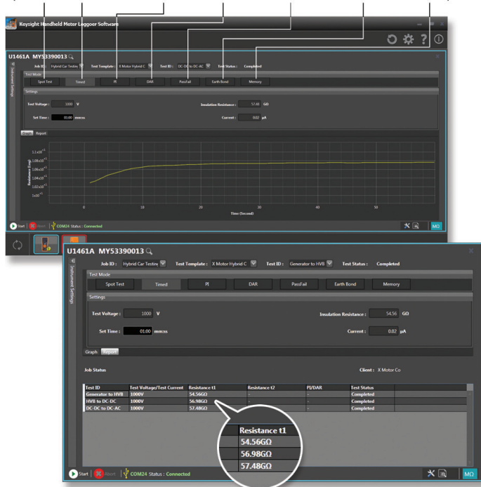
Figure 1. Keysight Handheld Logger Software Interface for Windows PC with guided operation and one button automatic report generation
