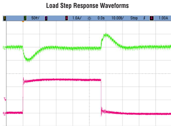
Figure 5. Load Step Response  $V_{IN} = 12V$ ,  $V_{OUT} = 1.8V$ , 2.5A Load Step (0A-2.5A)
