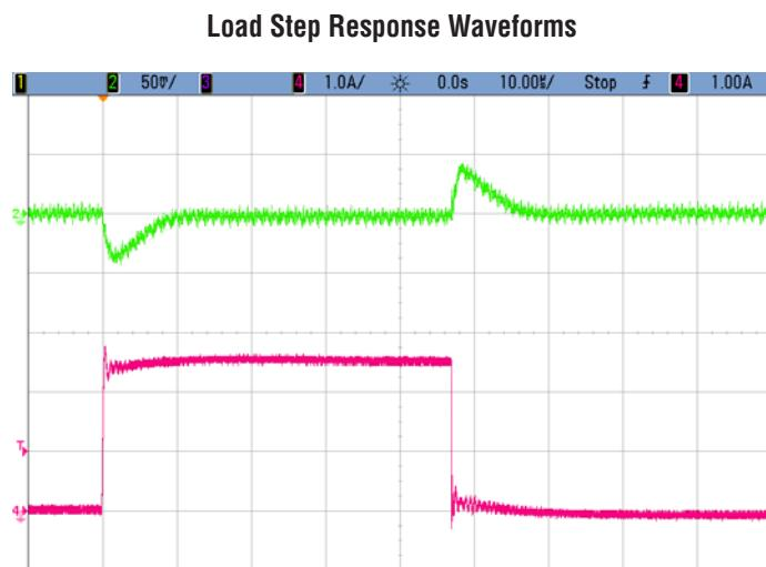
Figure 6. Load Step Response  $V_{IN} = 12V$ ,  $V_{OUT} = 3.3V$ , 2.5A Load Step (0A-2.5A)
