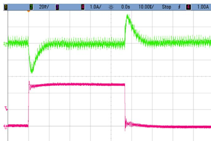
**Figure 4.** Load Step Response  $V_{IN} = 12V$ .  $V_{OUT} = 1.2V$ , 2.5A Load Step (0A-2.5A)
