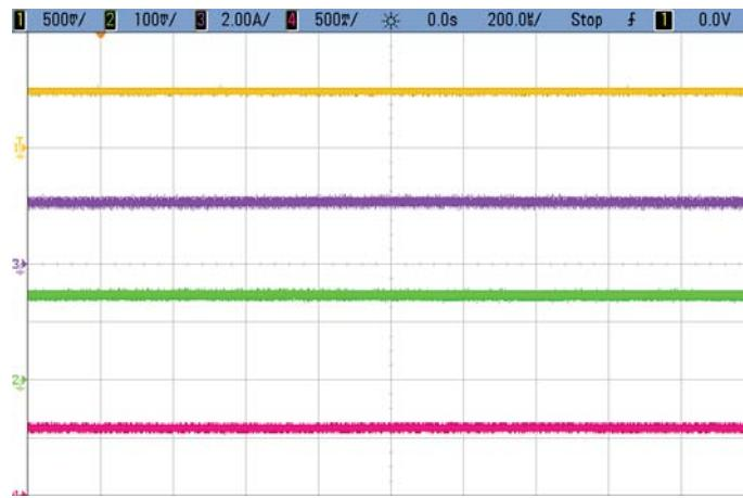
**Figure 7. Input and Output Current Monitoring**  $V_{IN} = 12V$ ,  $I_{IN} = 620mA$ ,  $V_{OUT} = 3.3V$ ,  $I_{OUT} = 2A$ ,  $f_{SW} = 1MHz$
