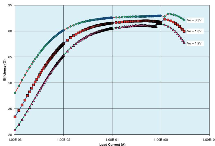
**Figure 8. Efficiency Graph**  $V_{IN} = 12V$ , Burst Mode,
