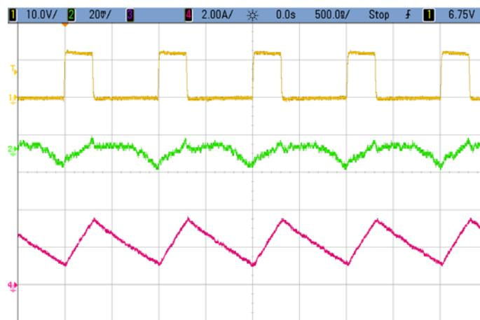
**Figure 3.** Switch Node Voltage, Output Ripple Voltage & Inductor Ripple Current Waveforms
