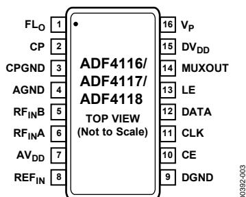
Figure 3. Pin Configuration
