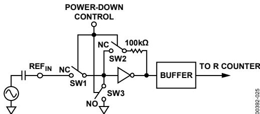
Figure 25. Reference Input Stage
