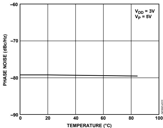
Figure 21. ADF4118 Phase Noise vs. Temperature
