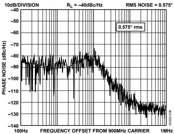
Figure 8. ADF4118 Integrated Phase Noise
