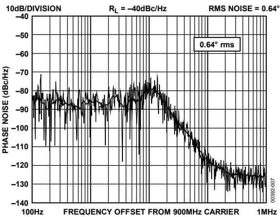
Figure 7. ADF4118 Integrated Phase Noise
