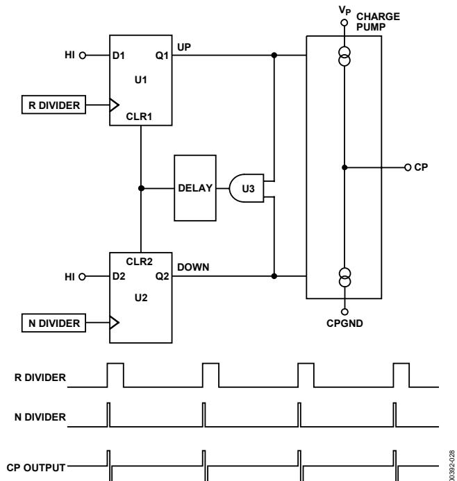
Figure 28. PFD Simplified Schematic and Timing (In Lock)
