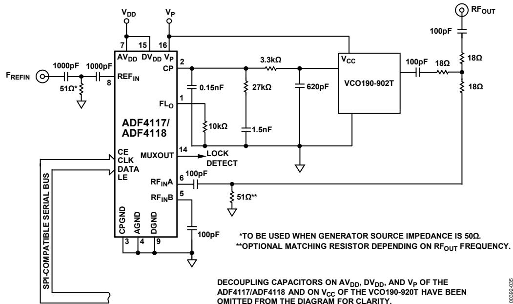
Figure 35. Local Oscillator for GSM Base Station
