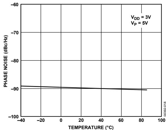
Figure 18. ADF4118 Phase Noise vs. Temperature
