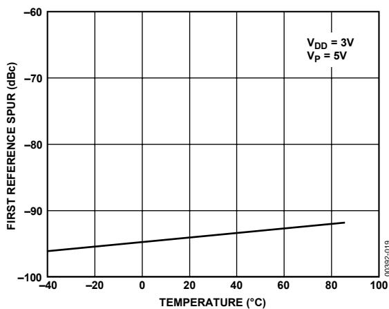
Figure 19. ADF4118 Reference Spurs vs. Temperature
