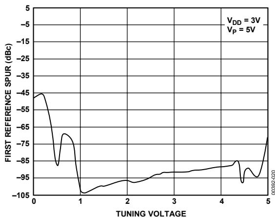
Figure 20. ADF4118 Reference Spurs (200 kHz) vs.  $V_{TUNE}$
