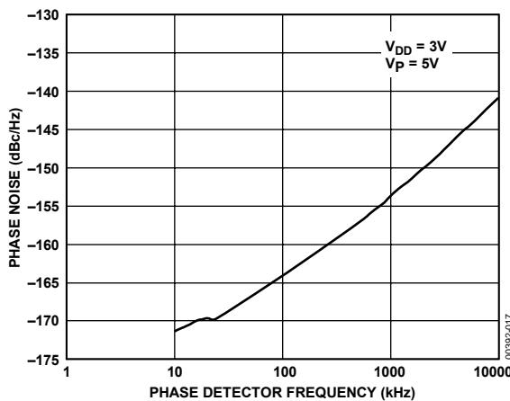
Figure 17. ADF4118 Phase Noise (Referred to CP Output) vs.
