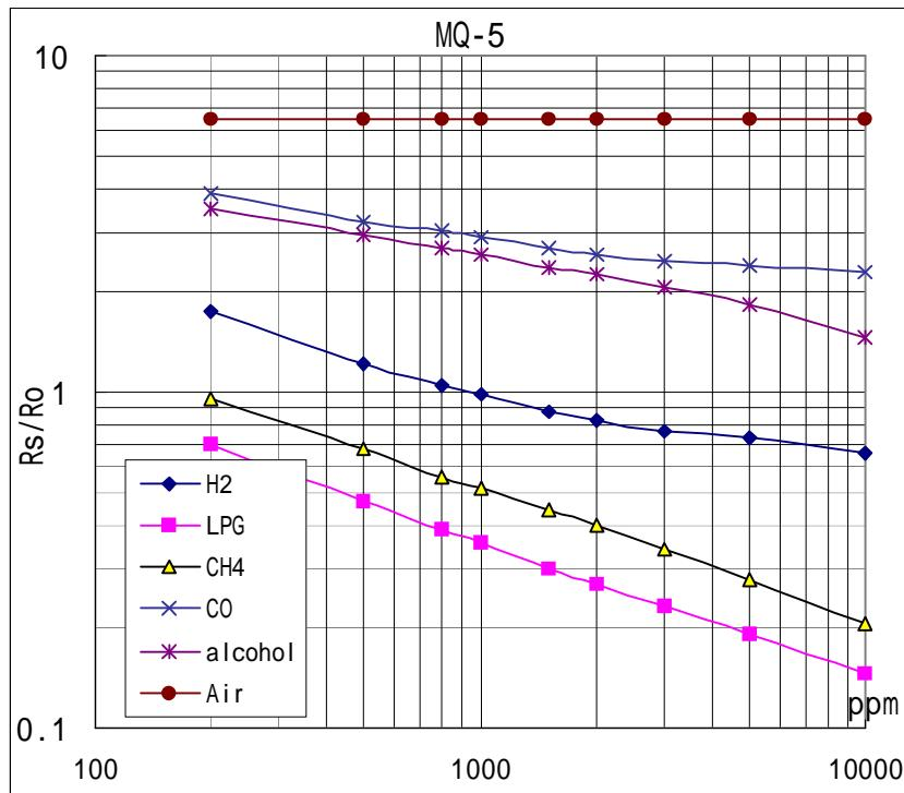
Fig.3 is shows the typical sensitivity characteristics of the MQ-5 for several gases.
