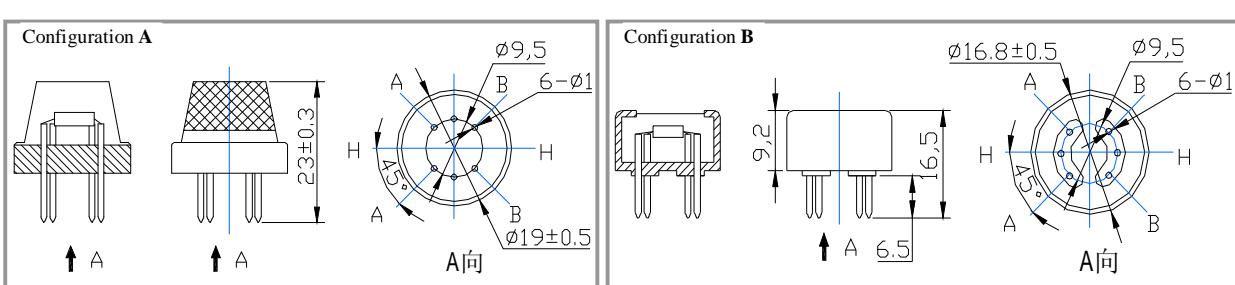
Structure and configuration of MQ-5 gas sensor is shown as Fig. 1 (Configuration A or B), sensor composed by
