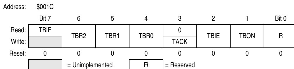
Figure 21-2. Timebase Control Register (TBCR)
