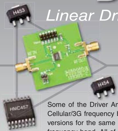
This Driver Amplifier Designer's Kit HMC-DK002 includes samples of 6 of Hittite's most popular GaAs InGaP HBT MMIC Amplifiers. The table below summarizes the features of each of the products included in this kit. Also included are 6 evaluation boards (assembled and tested), which enable the designer to immediately test each enclosed sample.
