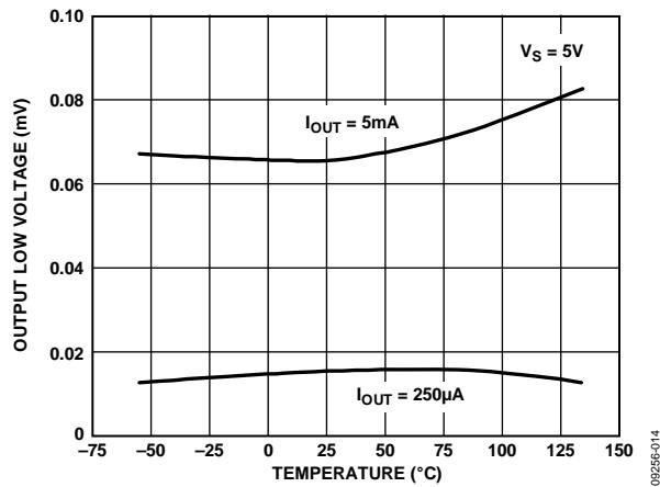
Figure 9. Output Low Voltage vs. Temperature
