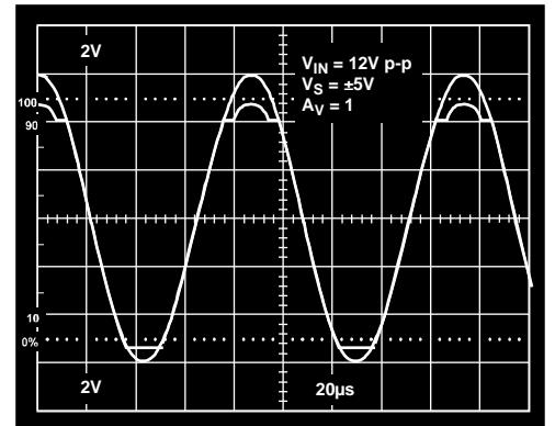
Figure 25. No Phase Reversal ( $V_{IN} = 12 V \text{ p-p}$ ,  $V_S = \pm 5 V$ ,  $A_V = 1$ )
