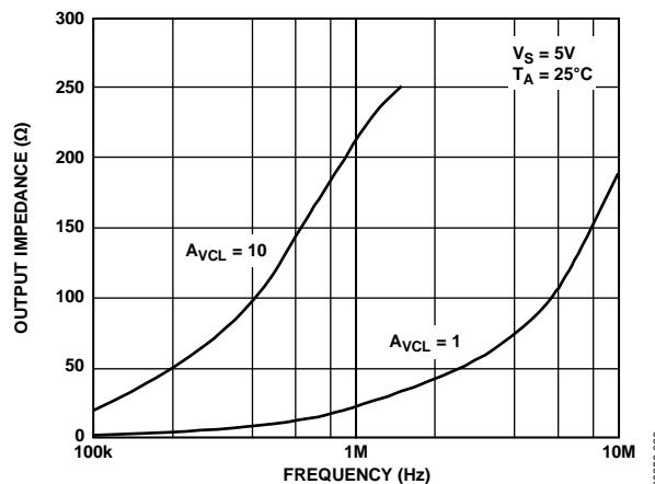
Figure 21. Output Impedance vs. Frequency
