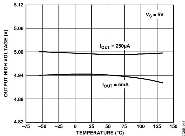
Figure 8. Output High Voltage vs. Temperature
