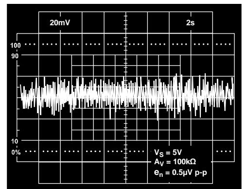
Figure 24. 0.1 Hz to 10 Hz Noise
