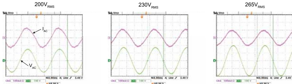
Line Voltage and Current at half load (350mA, 20V)
