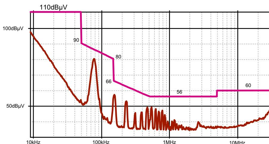
The performance graphs above were obtained from the board not having specific measures to suppress common mode emissions, such as inclusion of a common mode inductor in the AC line input circuitry. The above graphs show how shielding can significantly reduce emissions, particu-
