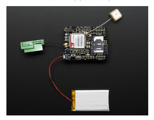
On its own, this shield can't do anything. It requires a microcontroller like an Arduino to drive it! You will also need some required accessories to make FONA work. **These are not included!**
