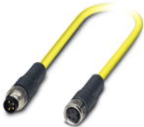
Sensor/Actuator cable, 4-position, PVC, Yellow RAL 1021, Plug straight M8, on Socket straight M8, Cable length: 0.5 m
