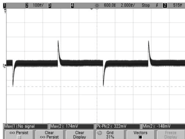
Step Load Transient Response (Vin=48V, Vout=nominal, Load=0, Iout=50 to 75 to 50% of full load, Ta=+25°C.) Trace 1=Vout, 100 mV/div., 2 mS/div.
