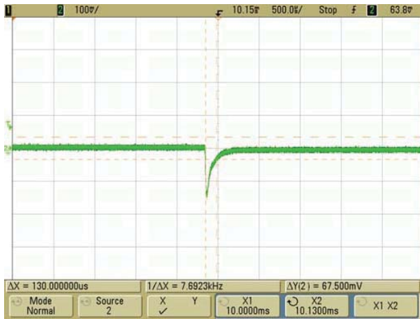
Step Load Transient Response (Slew=1A / \mu Sec., Vin=48V., Clod=0, Iout=22.5A to 15A)
