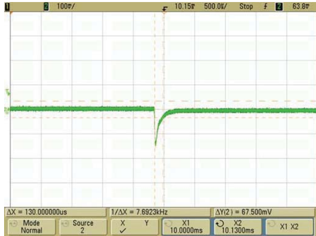
Step Load Transient Response (Slew=1A / \mu Sec., Vin=48V, Vout=nom., Iout=22.5A to 15A)
