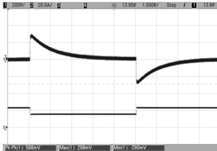
Step Load Transient Response ( V_{in} = 48V , V_{out} = \text{nom} , C_{load} = 1\mu F \parallel 10\mu F , I_{out} = 50 \text{ to } 75 \text{ to } 50\% of full load, T_a = +25^\circ C ) Ch1 = Vout, Ch2 = Iout.
