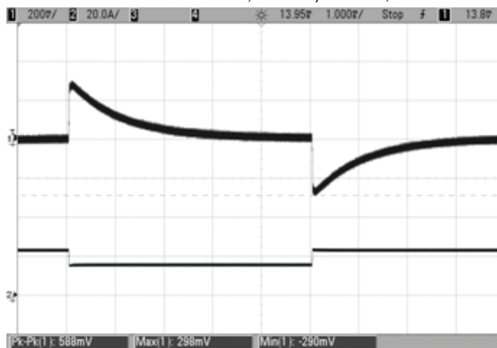
Step Load Transient Response ( V_{in} = 48V , V_{out} = \text{nom} , C_{load} = 1\mu F \parallel 10\mu F , I_{out} = 50 to 75 to 50\% of full load, T_a = +25^\circ C ) Ch1 = Vout, Ch2 = Iout.
