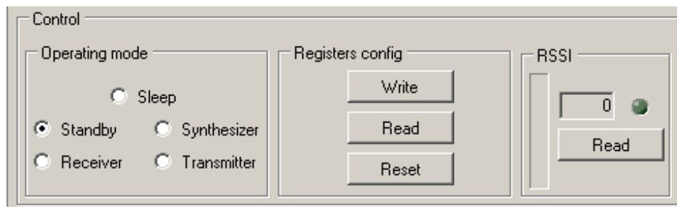
**Figure 13. The Mode Control Box also Incorporates RSSI**
