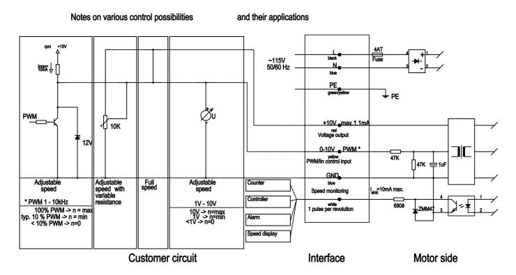
Not switchable via the supply voltage. Restart only after 5 minute delay via input voltage.
