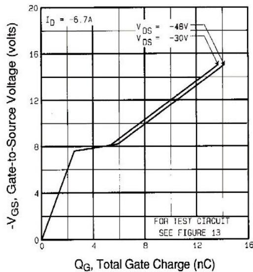
Fig. 6 - Typical Gate Charge vs. Gate-to-Source Voltage
