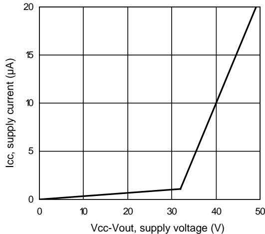
Figure 5 –  $I_{cc}$  off (µA) Vs  $V_{cc}-V_{out}$  (V)
