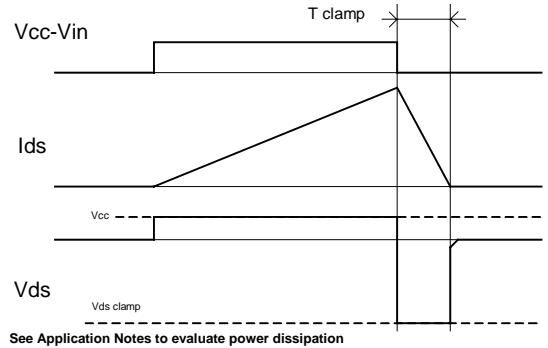
**Figure 2 – Active clamp waveforms**
