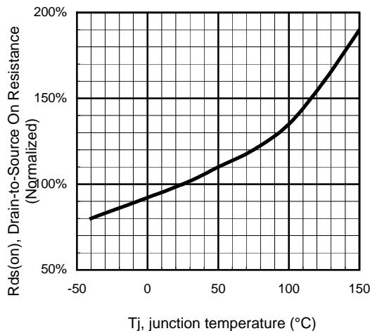
Figure 7 - Normalized  $R_{ds(on)}$  (%) Vs  $T_j$  (°C)
