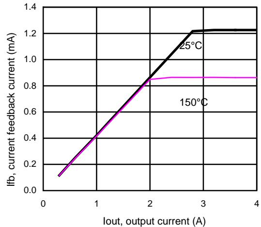
Figure 10 – Ifb (mA) Vs Iout (A)
