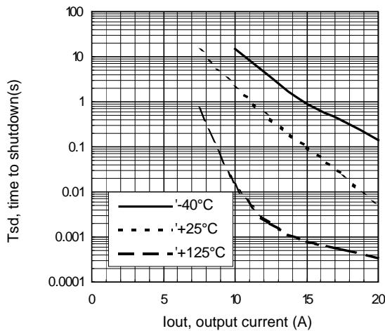
Figure 11 – Tsd (s) Vs Iout (A)
