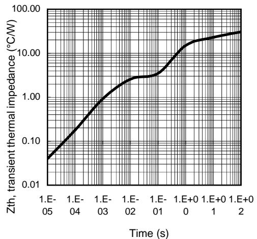
Figure 8 – Transient thermal impedance (°C/W) Vs time (s)
