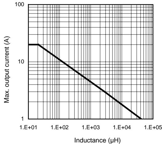
Figure 9 – Max. Iout (A) Vs inductance ( $\mu\text{H}$ )
