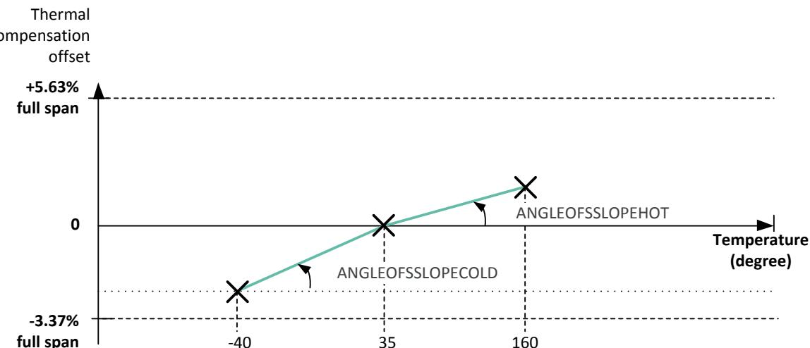
Figure 10 - Input range from -40Deg.C up to 160 Deg.C
