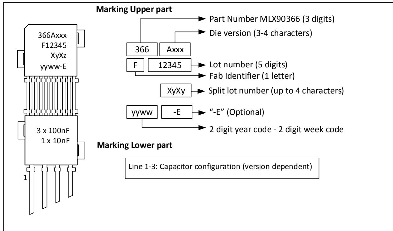
Figure 15 – DMP-4 marking and pinout convention
