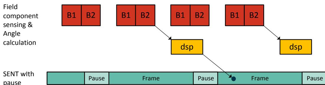
Figure 4 - Latency - Case FILTER = 0 (not recommended)
