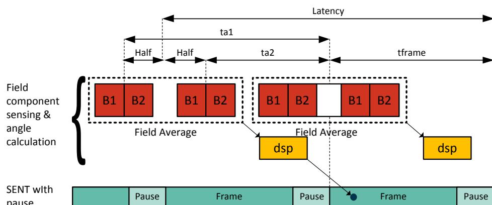
Figure 3 - Latencies (acquisition to output delays) – FILTER = 1 (recommended)
