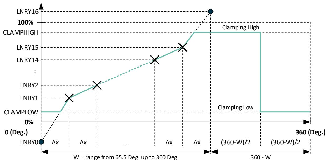
Figure 9 - Input range from 65.5Deg. up to 360Deg.
