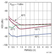
HD3 at 140MHz vs V<sub>CM</sub> Over Temperature
