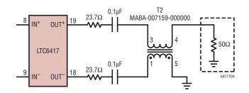
Figure 4. Output Termination for Differential 50  $\Omega$  Load Using a 1:1 Balun
