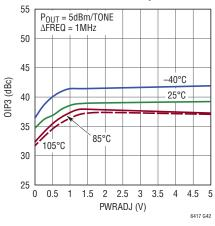
OIP3 at 500MHz vs PWRADJ Over Temperature
