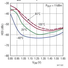
HD3 at 700MHz vs PWRADJ Over Temperature
