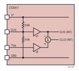
Figure 7. Internal Circuitry Generating Symmetric Clamp Voltages with Respect to V<sub>CM</sub>
