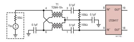
Figure 2. Input Termination for Differential 50 $\Omega$  Input Impedance Using a 1:4 Balun
