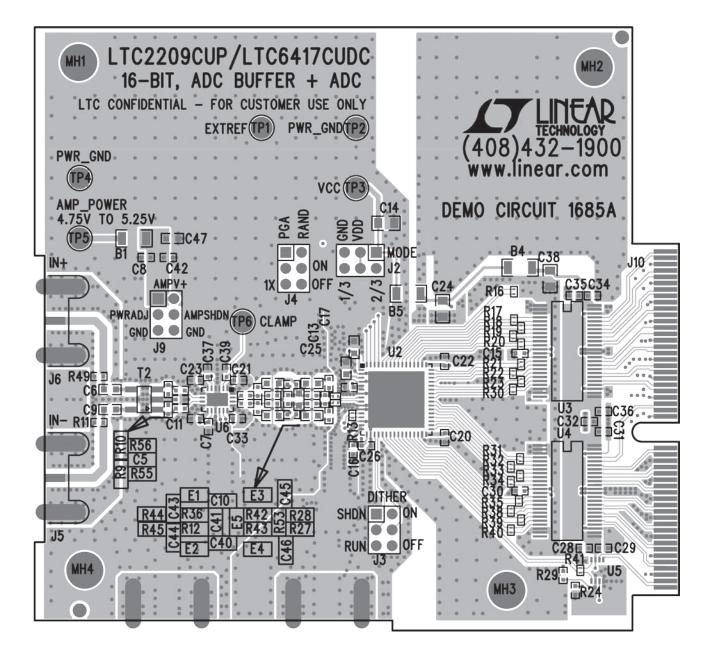
Figure 18. Demo Board DC1685A Layout
