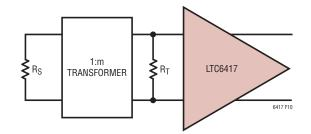
Figure 10. LTC6417 with a Transformer
