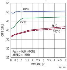
OIP3 at 140MHz vs PWRADJ Over Temperature
