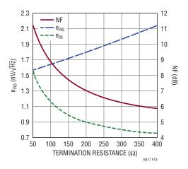
Figure 13. LTC4617 Output and Input Noise Density and NF vs Termination Resistance
