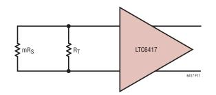
Figure 11. Source Resistance Referred to the Secondary
