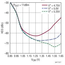
HD3 at 500MHz vs PWRADJ Over Temperature
