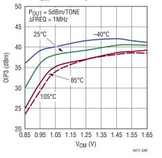
OIP3 at 500MHz vs V<sub>CM</sub> Over Temperature
