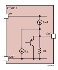
Figure 9. LTC6417 Internal Topology Showing V<sub>OR</sub> Pin with Pull-Down Resistor and Clamp
