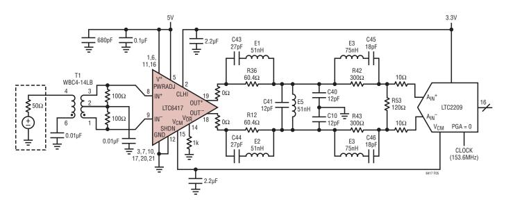
Figure 5. DC1685A Simplified Schematic with Suggested Bandpass Filter for Driving an LTC2209 16-Bit ADC at 140MHz
