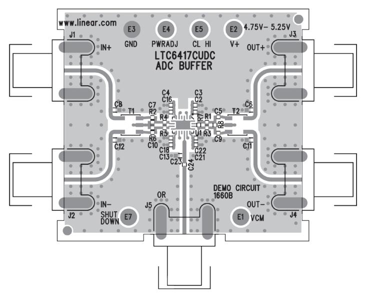
Figure 16. Demo Board DC1660B Layout
