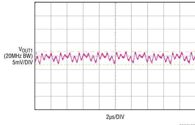
**Figure 5. Output Voltage Ripple at  $V_{IN} = 12V$ ,
