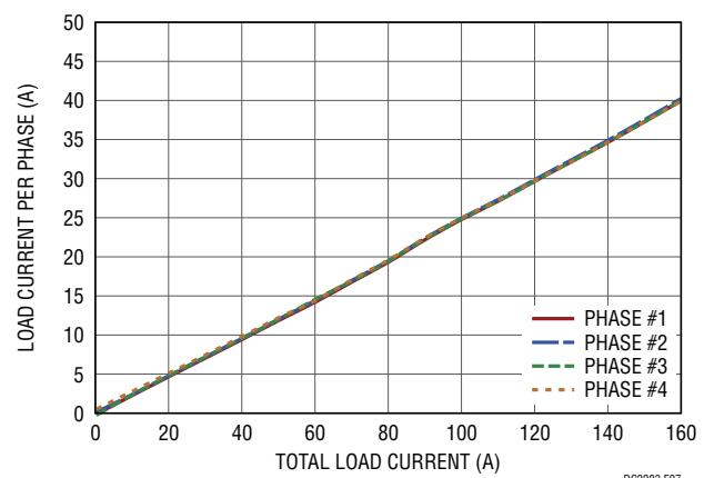
**Figure 7. Current Sharing vs Load Current
