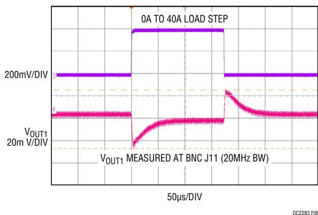
**Figure 6. Transient Response at  $V_{IN} = 12V$ ,
