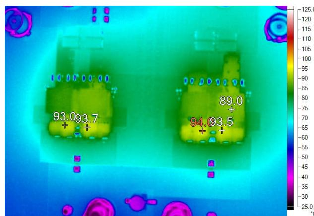
**Figure 8. Thermal Performance at  $V_{IN} = 12V$ ,  $V_{OUT1} = 1V$ ,
