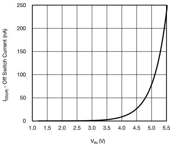
Fig. 10 - Off Switch Current vs. Input Voltage
