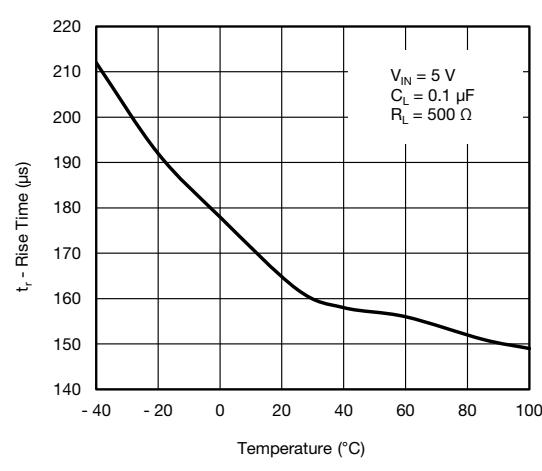
Fig. 15 - Rise Time vs. Temperature
