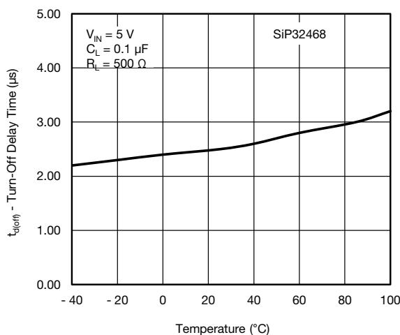
Fig. 18 - Turn-off Delay Time vs. Temperature
