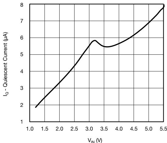
Fig. 4 - Quiescent Current vs. Input Voltage
