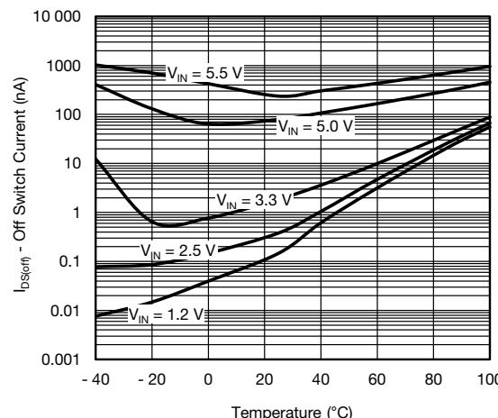
Fig. 13 - Off Switch Current vs. Temperature
