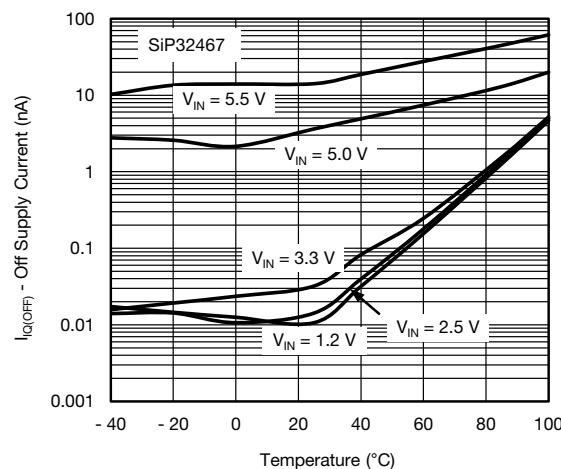
Fig. 9 - Off Supply Current vs. Temperature
