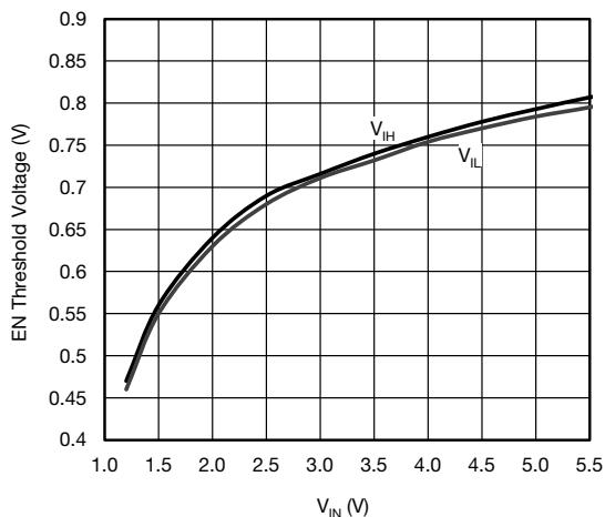
Fig. 17 - EN Threshold Voltage vs. Input Voltage
