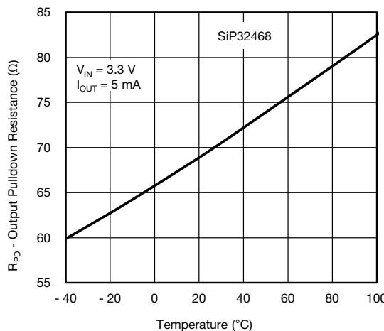
Fig. 20 - Output Pulldown Resistance vs. Temperature
