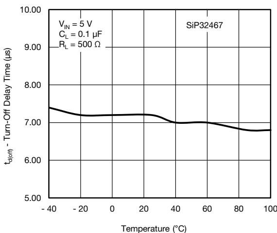
Fig. 21 - Turn-off Delay Time vs. Temperature
