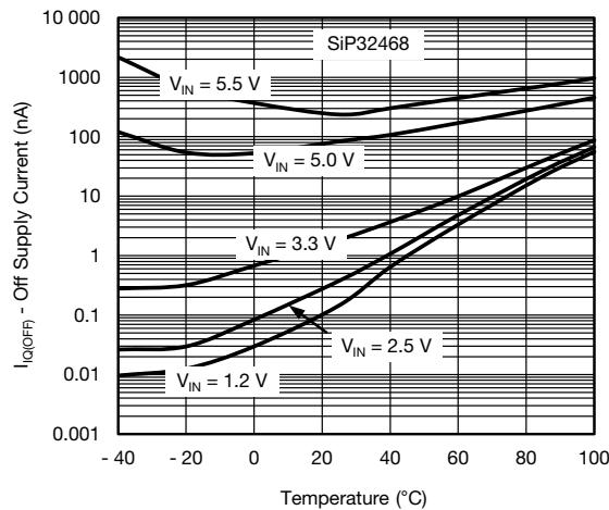
Fig. 6 - Off Supply Current vs. Temperature
