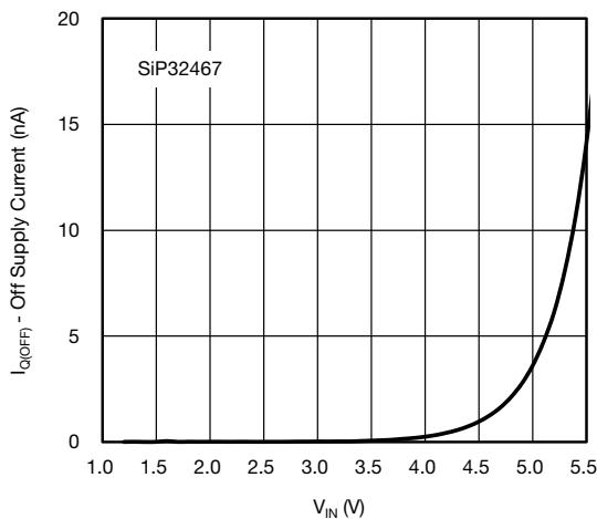
Fig. 8 - Off Supply Current vs. Input Voltage
