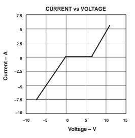
NOTE A: Typical current versus voltage curve was derived using the IEC 1.2/50-µs surge waveform.
