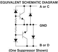
NOTE: All GND terminals should be connected to ground.
