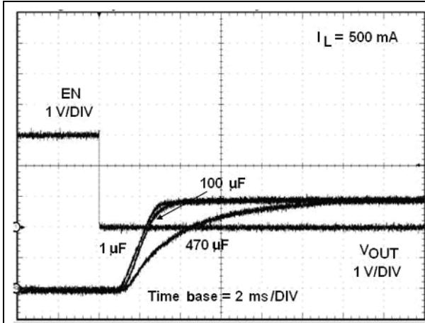
**Figure 8.** Voltage output turn-off delay time
