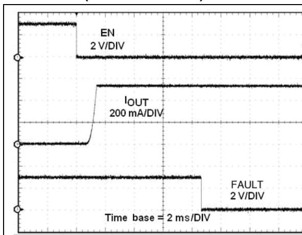
Figure 39. OC protection at  $V_{OUT} = 3.0 (STMPs2161/2171- detail)$
