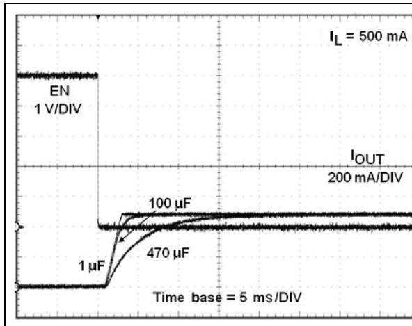
**Figure 6.** Current output turn-off delay time (STMPS2141/2151, 5 V)
