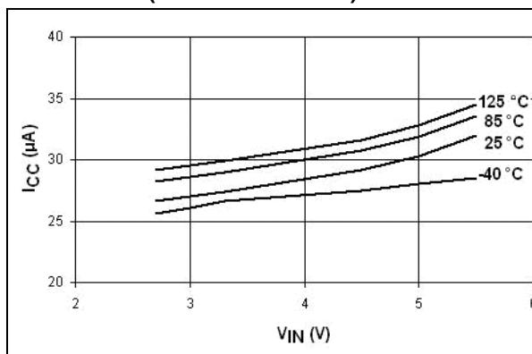
**Figure 43.**  $I_{CC}$  vs. temperature (enabled)
