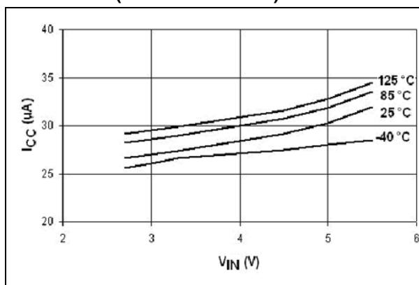
**Figure 18.**  $I_{CC}$  vs. temperature (enabled)
