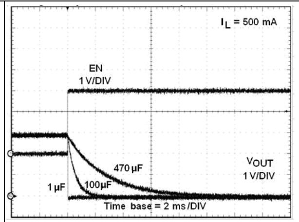
**Figure 9.** Current output turn-on delay time
