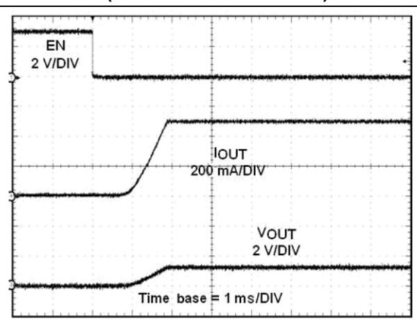
**Figure 40.** OC protection at  $V_{OUT} = 5.0$  V
