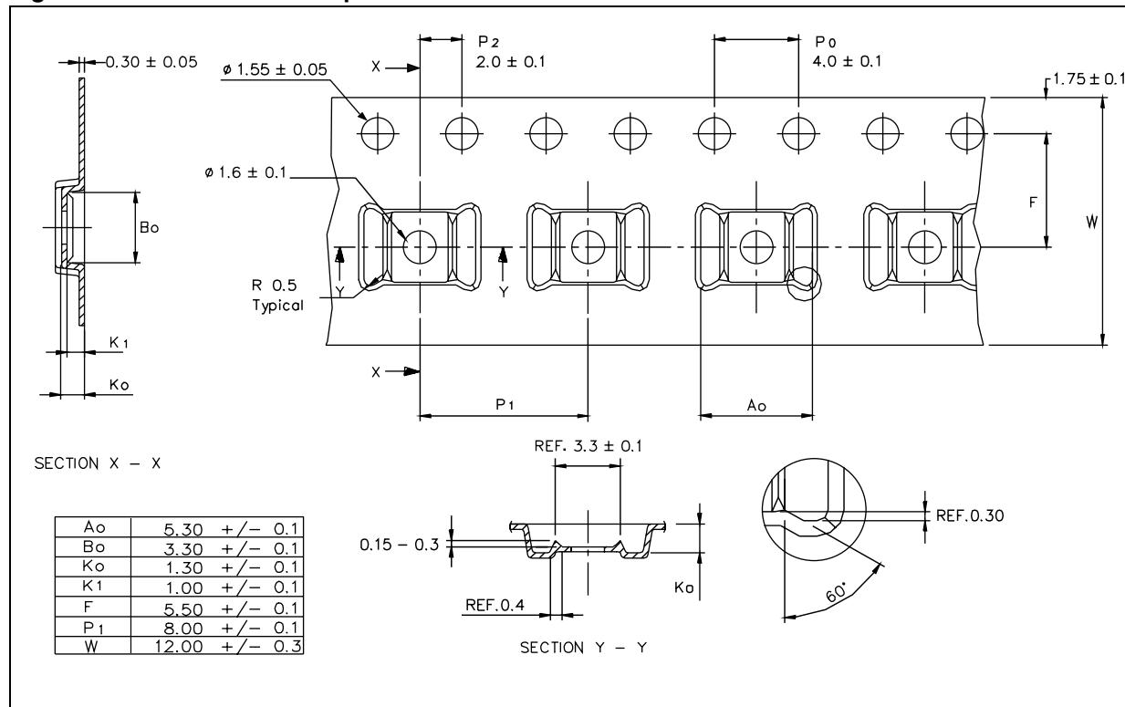
**Figure 60.** Reel information
