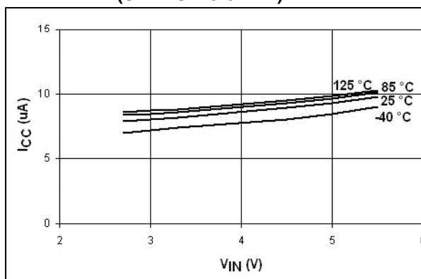
**Figure 45.**  $I_{CC}$  vs. temperature (disabled)
