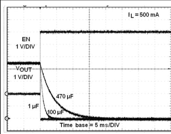
**Figure 30. Current output turn-on delay time (STMPS2161/2171, 5 V)**
