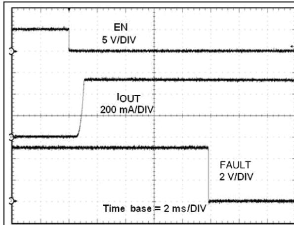
**Figure 41.** OC protection at  $V_{OUT} = 5.0$  V
