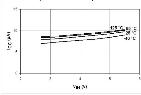
**Figure 20.**  $I_{CC}$  vs. temperature (disabled)
