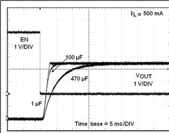
**Figure 29. Voltage output turn-off delay time (STMPS2161/2171, 5 V)**
