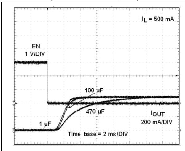
**Figure 10.** Current output turn-off delay time
