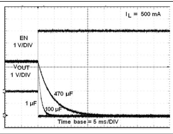
**Figure 5.** Current output turn-on delay time (STMPS2141/2151, 5 V)
