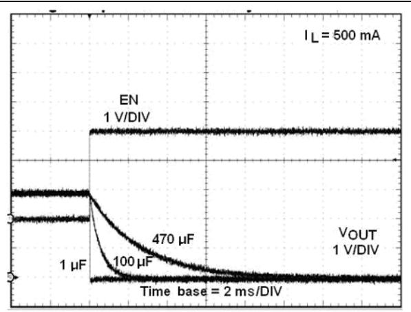
Figure 34. Current output turn-on delay time
