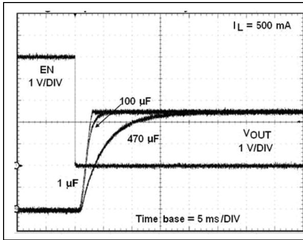
**Figure 4.** Voltage output turn-off delay time (STMPS2141/2151, 5 V)
