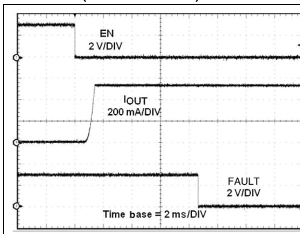
Figure 14. OC protection at V<sub>OUT</sub> = 3.0 V
