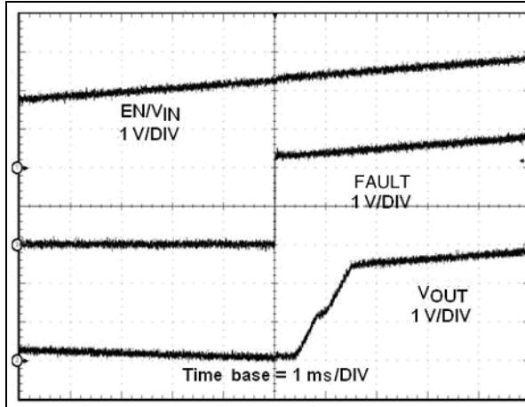
Figure 37. UVLO falling (STMPs2161/2171)
