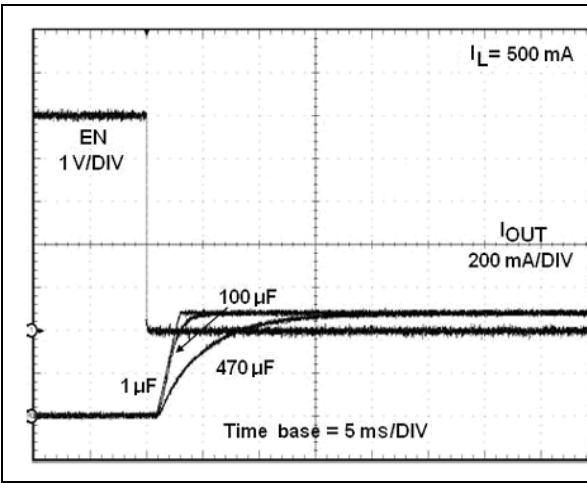
**Figure 31. Current output turn-off delay time (STMPS2161/2171, 5 V)**
