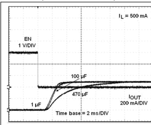
Figure 35. Current output turn-off delay time
