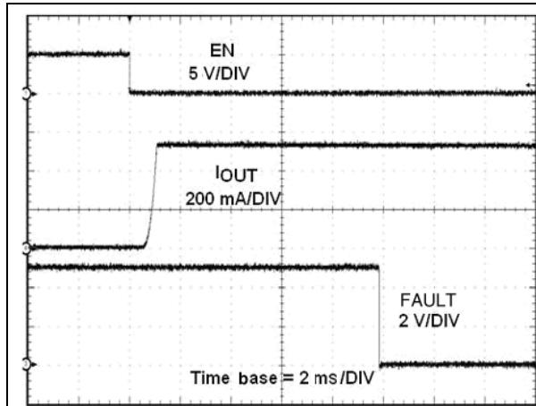
**Figure 16.** OC protection at  $V_{OUT} = 5.0$  V
