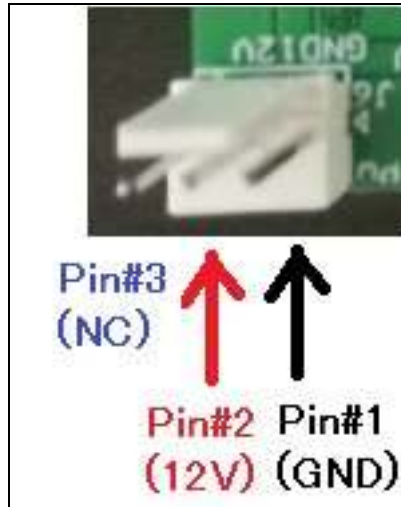
Figure-5: J6 connector for fan power supply
