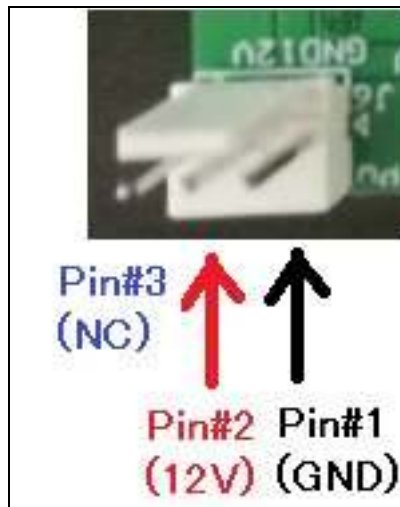
Figure-5: J6 connector for fan power supply
