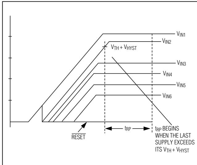
Figure 4. *RESET* Output with Various Input Voltages
