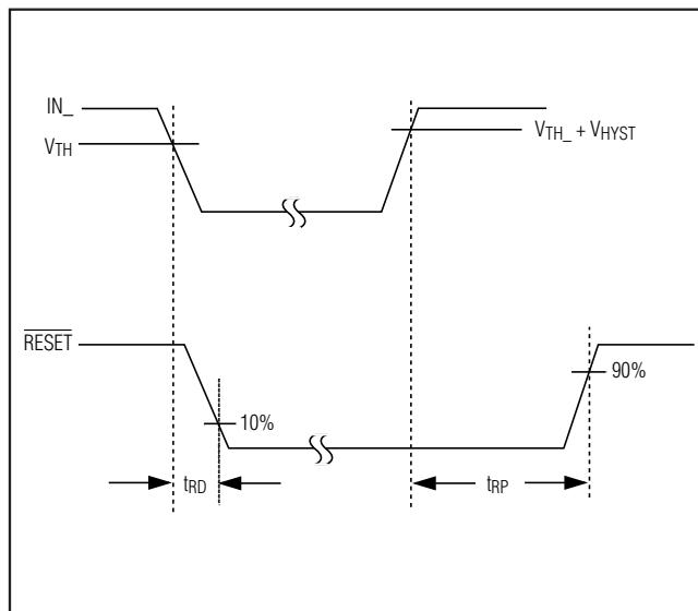
Figure 2. RESET Output Timing Diagram
