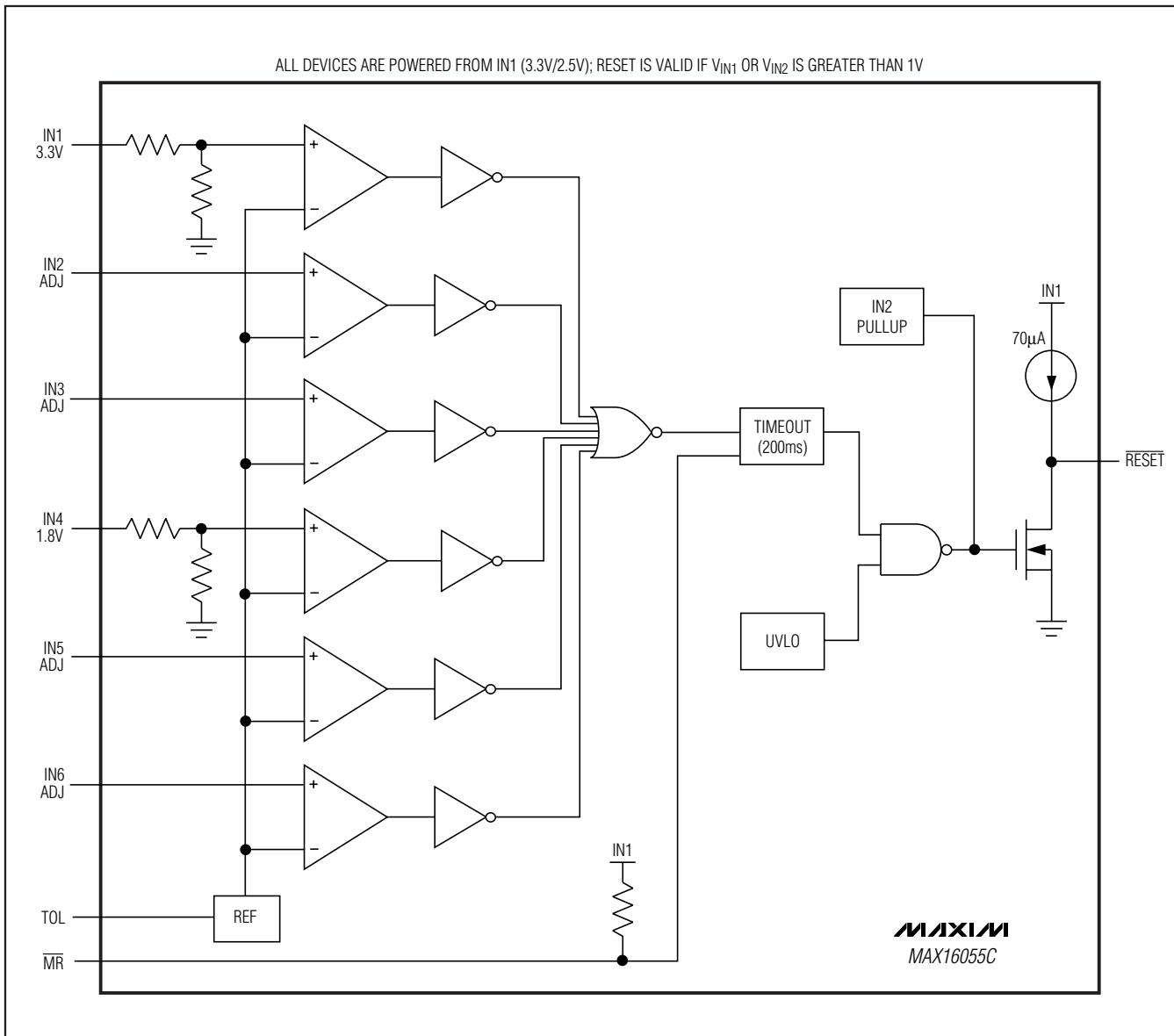
Figure 1. Functional Diagram
