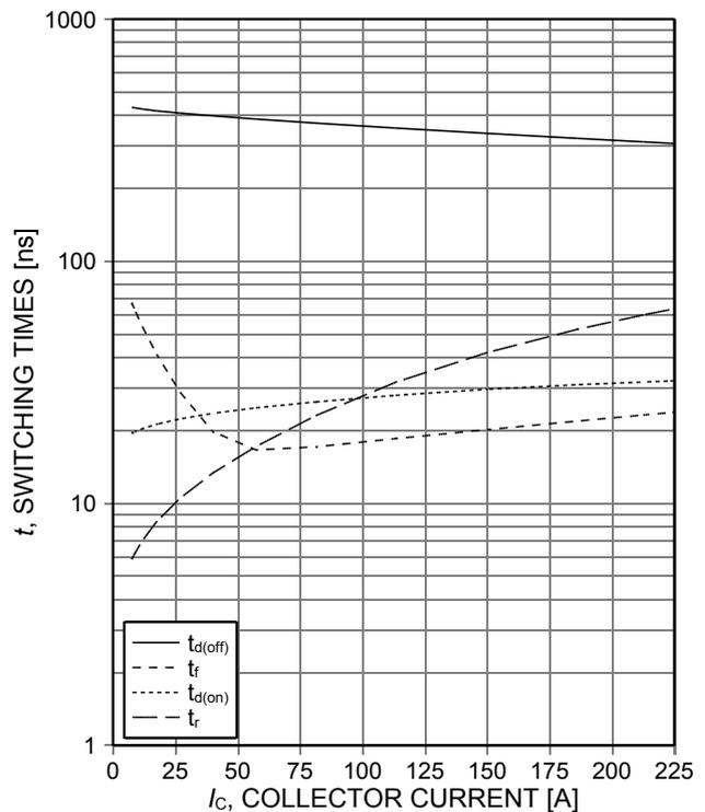
Figure 8. Typical switching times as a function of collector current (inductive load,  $T_{vj}=150^{\circ}\text{C}$ ,  $V_{CE}=400\text{V}$ ,  $V_{GE}=0/15\text{V}$ ,  $R_{G(on)}=10\Omega$ ,  $R_{G(off)}=18\Omega$ , dynamic test circuit in Figure E)
