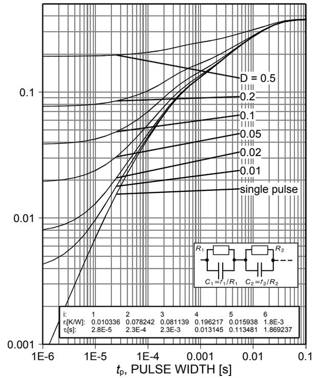
Figure 18. IGBT transient thermal impedance ( $D=t_p/T$ )
