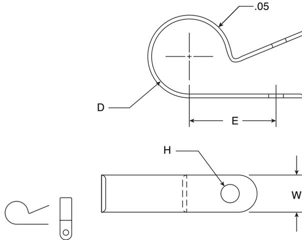
Molded nylon cable clamps secure, insulate, and route cable, wiring, tubing, piping, and fiber optics. These tough, durable, chemical resistant Nylon 6/6 cable clamps are perfect for applications in electronics, automotive, air craft, appliance, and many other industries.
