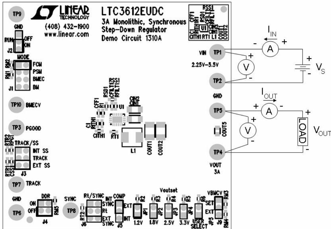
**Figure 1. Proper Equipment Measurement Set-Up**
