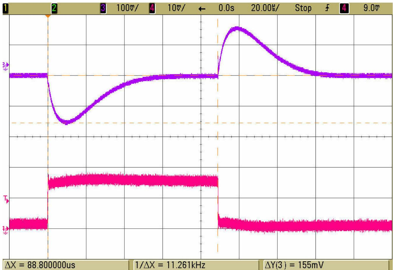
**Figure 4. Load Step Response**
