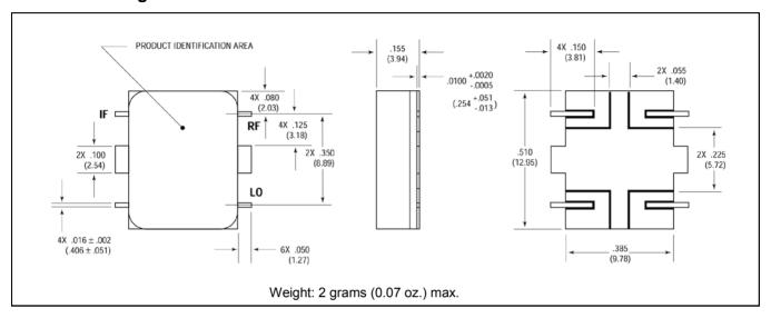
\* Dimensions are inches (millimeters) ±0.015 (0.38) unless otherwise specified.
