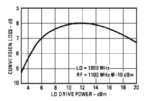
Conversion Loss vs. Drive Level: The minimum recommended drive level is +7 dBm. The maximum recommended drive level is +18 dBm.
