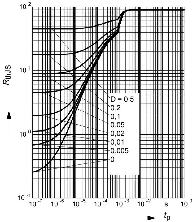
**Permissible Pulse Load  $I_{Fmax}/I_{FDC} = f(t_p)$**
