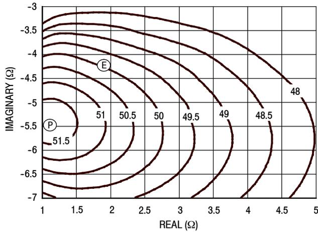
Figure 33. P3dB Load Pull Output Power Contours (dBm)
