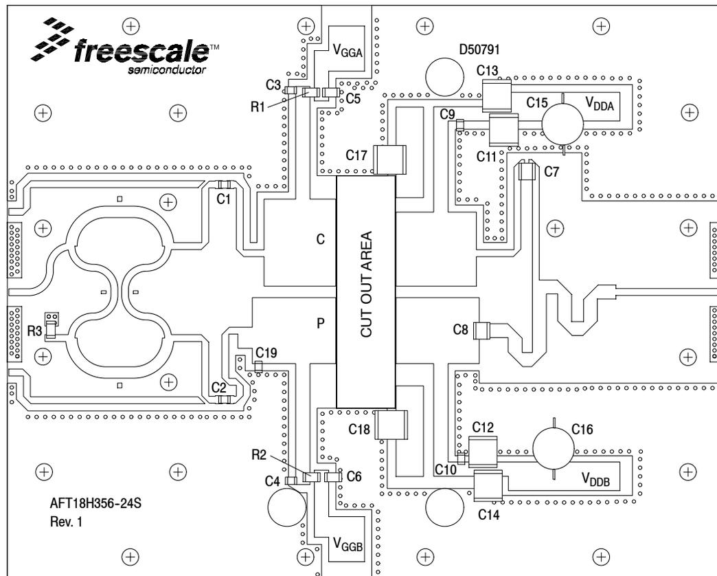
Figure 3. AFT18H356-24SR6 Characterization Test Circuit Component Layout — 1805–1880 MHz
