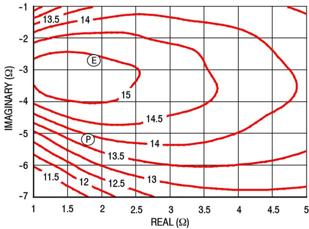
Figure 39. P1dB Load Pull Gain Contours (dB)
