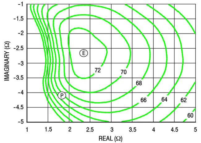
Figure 22. P3dB Load Pull Efficiency Contours (%)
