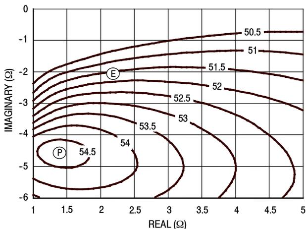
Figure 17. P1dB Load Pull Output Power Contours (dBm)
