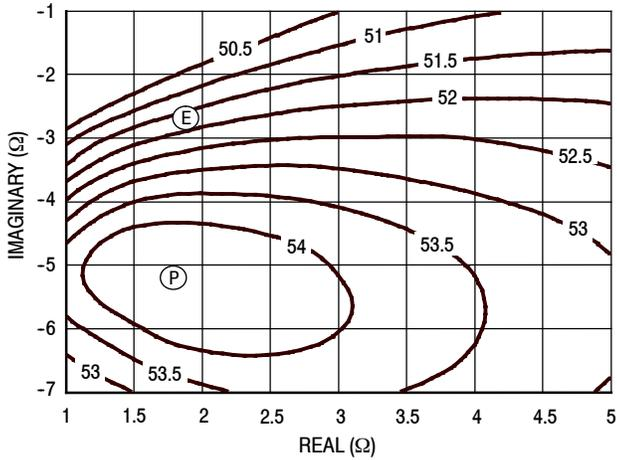
Figure 37. P1dB Load Pull Output Power Contours (dBm)
