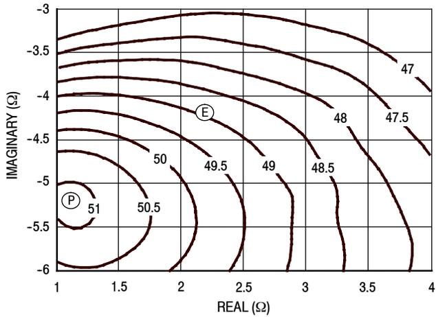
Figure 29. P1dB Load Pull Output Power Contours (dBm)
