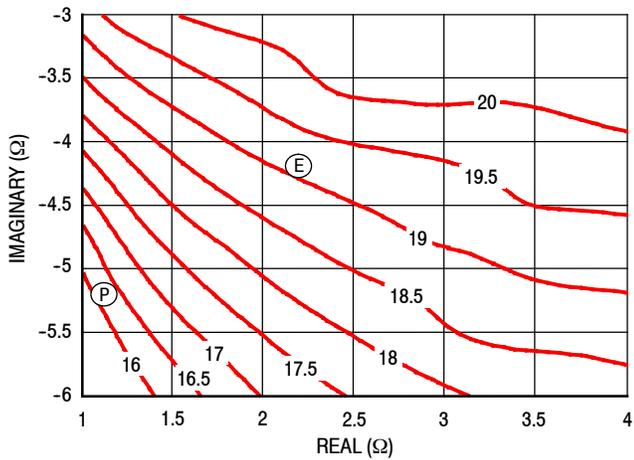
Figure 31. P1dB Load Pull Gain Contours (dB)
