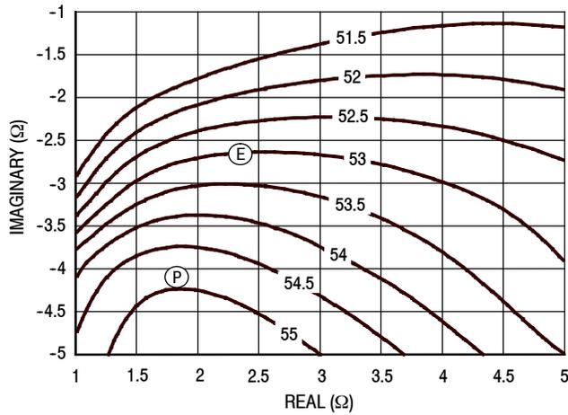
Figure 21. P3dB Load Pull Output Power Contours (dBm)
