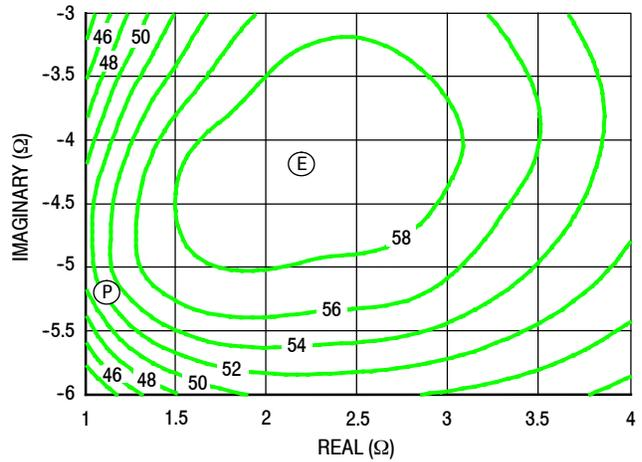
Figure 30. P1dB Load Pull Efficiency Contours (%)
