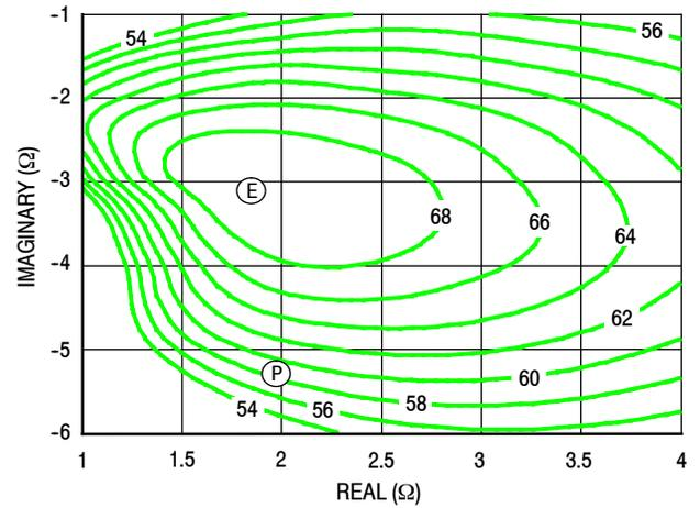
Figure 42. P3dB Load Pull Efficiency Contours (%)
