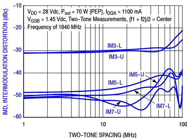
**Figure 5. Intermodulation Distortion Products versus Two-Tone Spacing**
