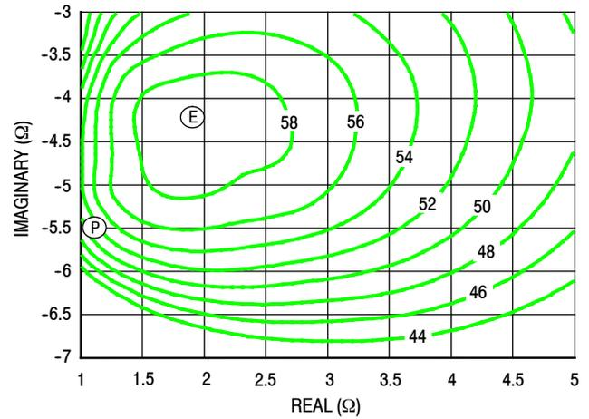
Figure 34. P3dB Load Pull Efficiency Contours (%)
