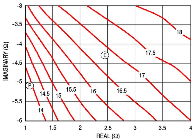
**Figure 15. P3dB Load Pull Gain Contours (dB)**
