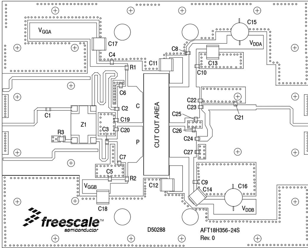
Figure 2. AFT18H356-24SR6 Production Test Circuit Component Layout — 1805–1880 MHz
