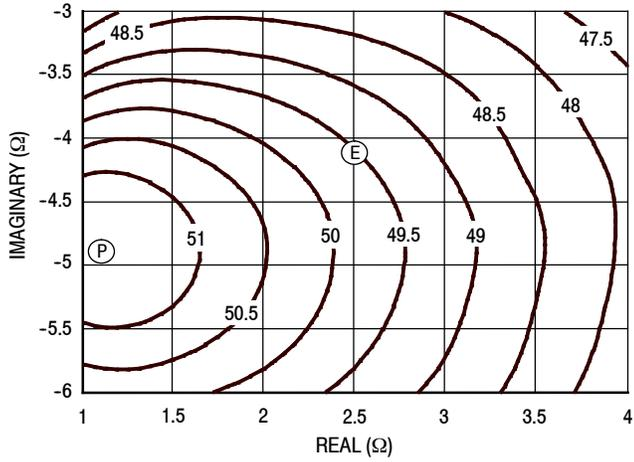
**Figure 9. P1dB Load Pull Output Power Contours (dBm)**
