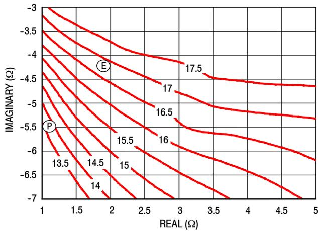
Figure 35. P3dB Load Pull Gain Contours (dB)
