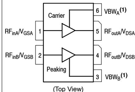
Figure 1. Pin Connections
