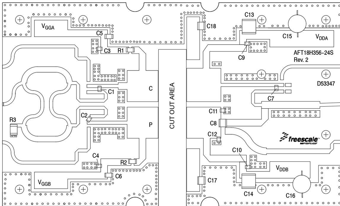
**Figure 25. AFT18H356-24SR6 Test Circuit Component Layout — 1930–1995 MHz**
