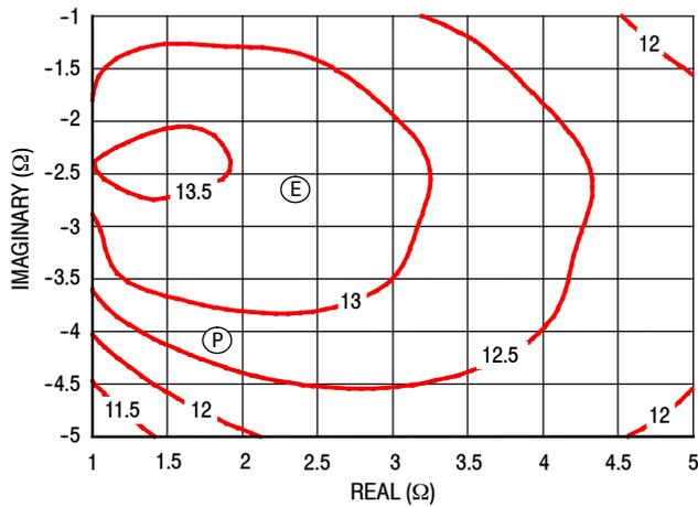
Figure 23. P3dB Load Pull Gain Contours (dB)
