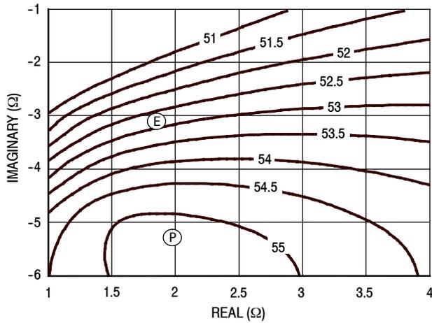
Figure 41. P3dB Load Pull Output Power Contours (dBm)
