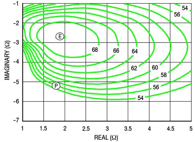
Figure 38. P1dB Load Pull Efficiency Contours (%)
