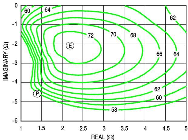
Figure 18. P1dB Load Pull Efficiency Contours (%)
