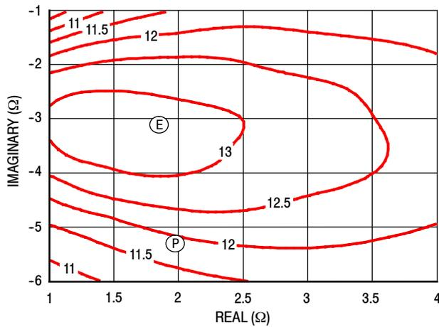
Figure 43. P3dB Load Pull Gain Contours (dB)
