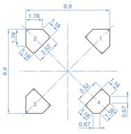
The positive polarity terminal: 1 The negative polarity terminal: 2=3=4 common Dimensions in mm
