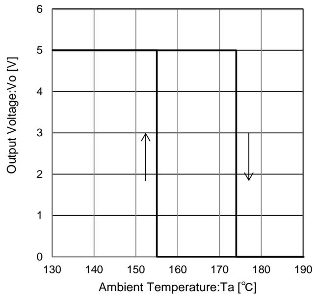
Figure 15. Thermal Shutdown
