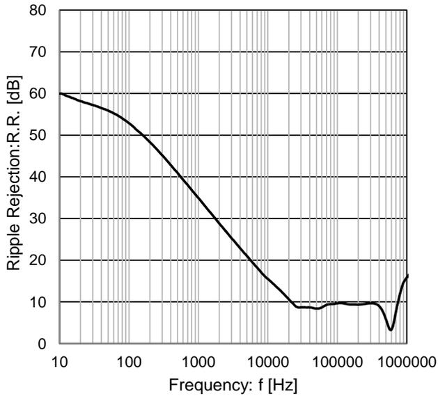
Figure 10. Ripple Rejection
