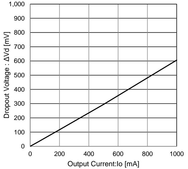
Figure 9. Dropout Voltage
