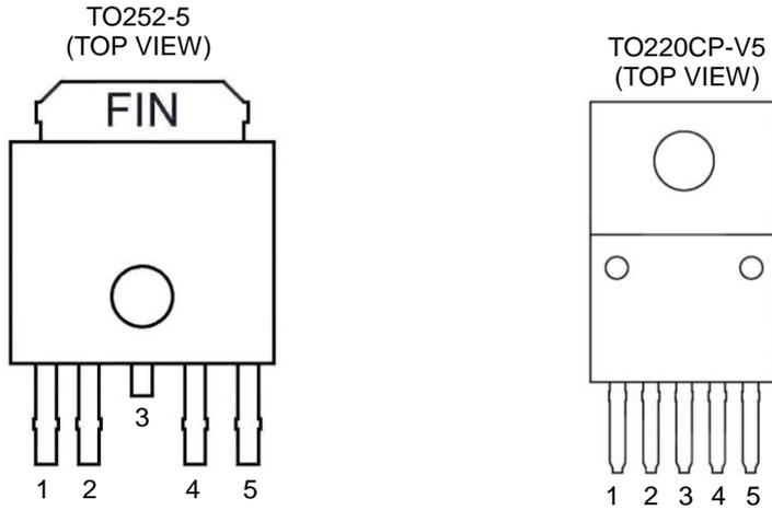
Figure 2. Pin Configurations
