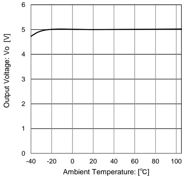
Figure 11. Output Voltage
