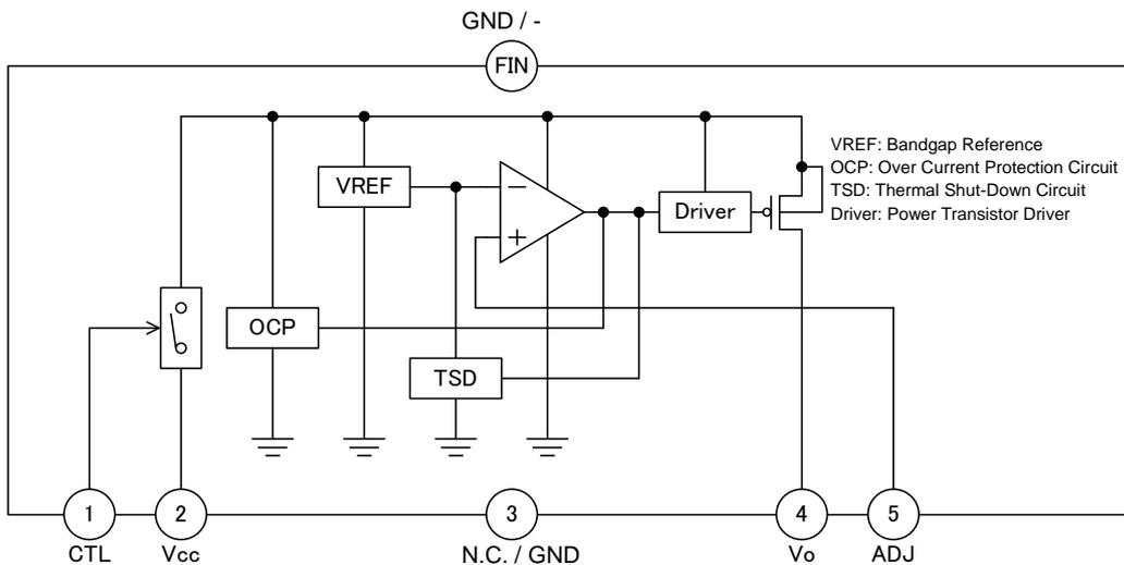
Figure 3. Block Diagram
