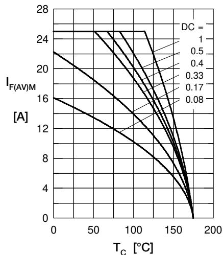
Fig. 5 Max. forward current vs. case temperature
