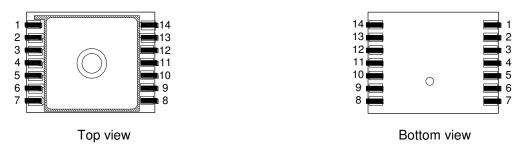
Fig. 2: Pin configuration of MS5536-CPJU, MS5536-CNJU
