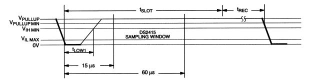
$60~\mu s \leq t_{SLOT} < 120~\mu s$   $1~\mu s \leq t_{LOW1} < 15~\mu s$   $1~\mu s \leq t_{REC} < \infty$
