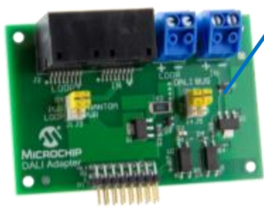
DALI Adapter with 2-wire & RJ45 connections
