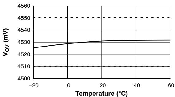
Figure 9.  $V_{OV}$  vs. Temperature
