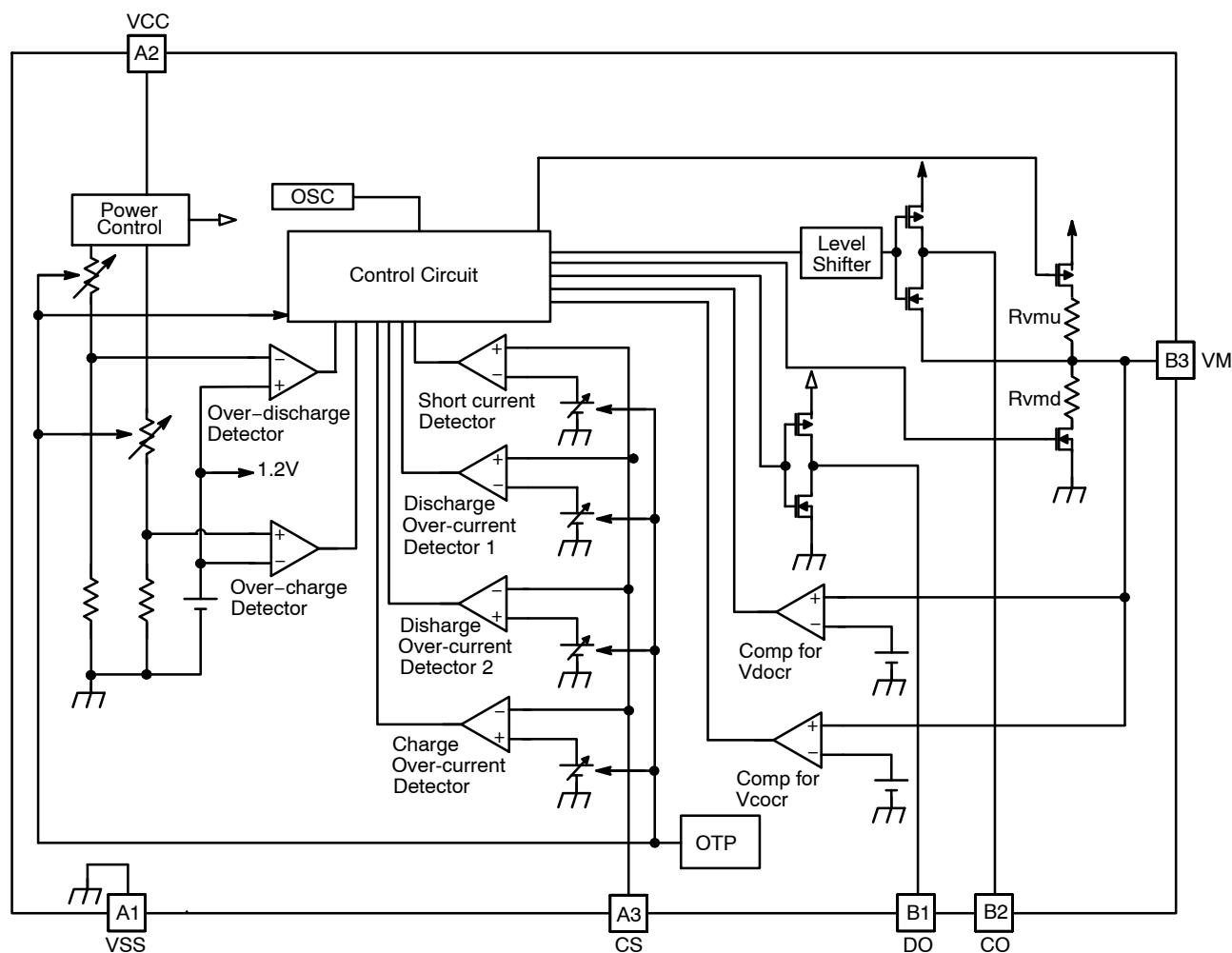
**Figure 4. Block Diagram**
