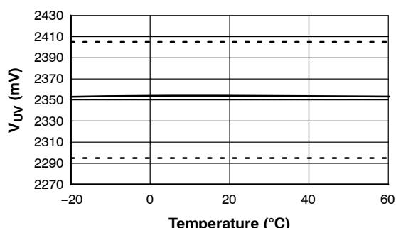
Figure 10.  $V_{UV}$  vs. Temperature
