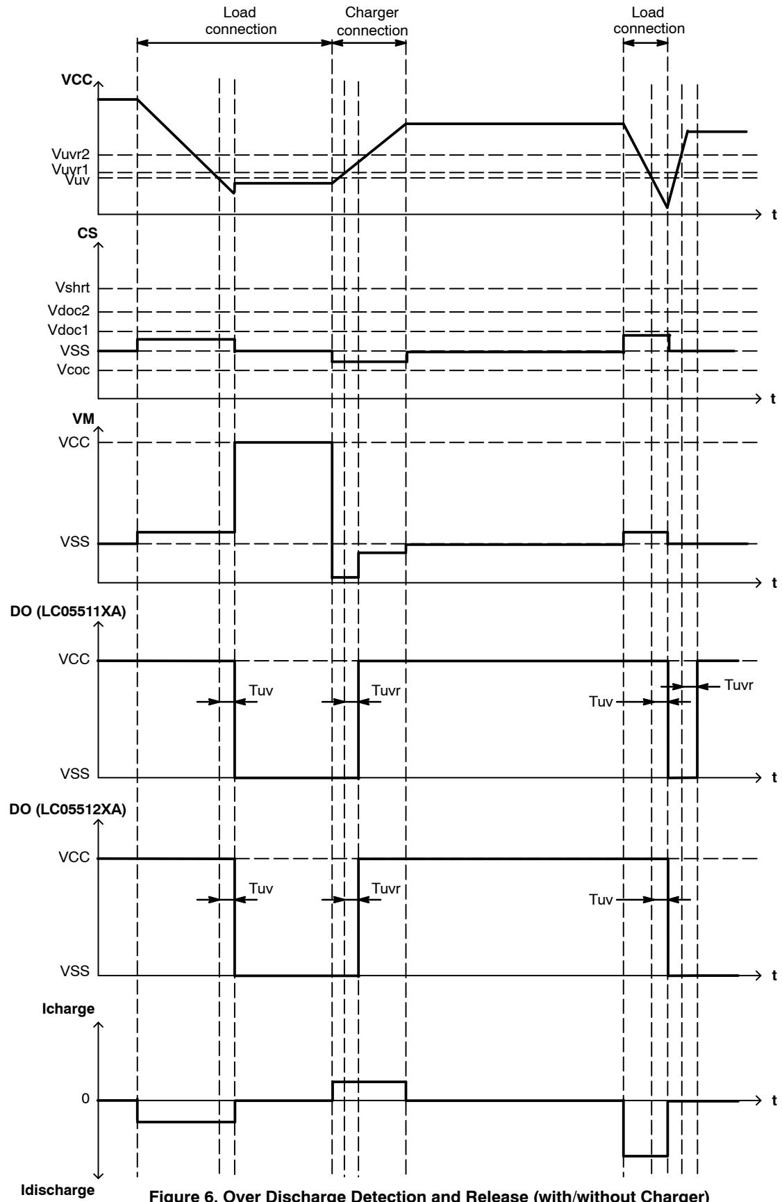
Figure 6. Over Discharge Detection and Release (with/without Charger)
