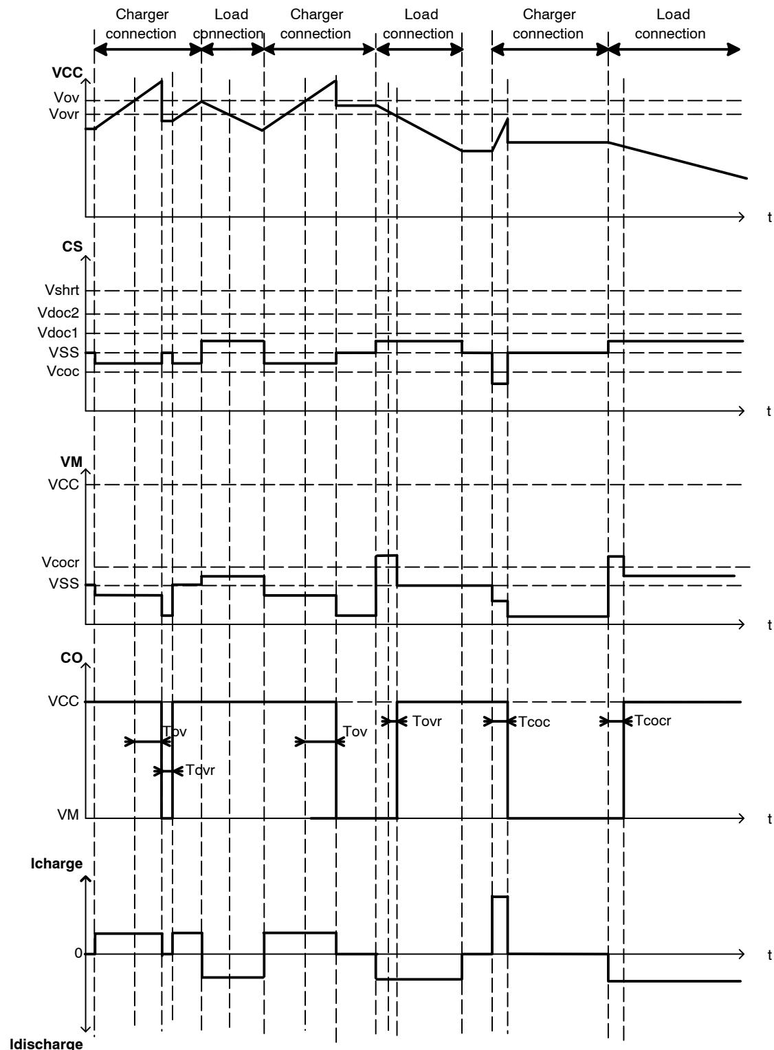
Figure 5. Over Charge Voltage and Charge Over Current
