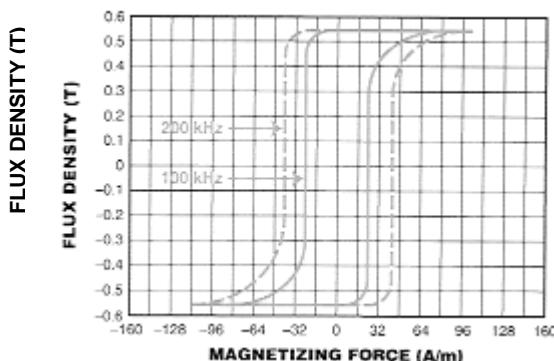
METGLAS® Square Loop magnetic cores are specifically designed to exhibit an extremely square dc Hysteresis loop and high BSAT resulting in the following important benefits:
